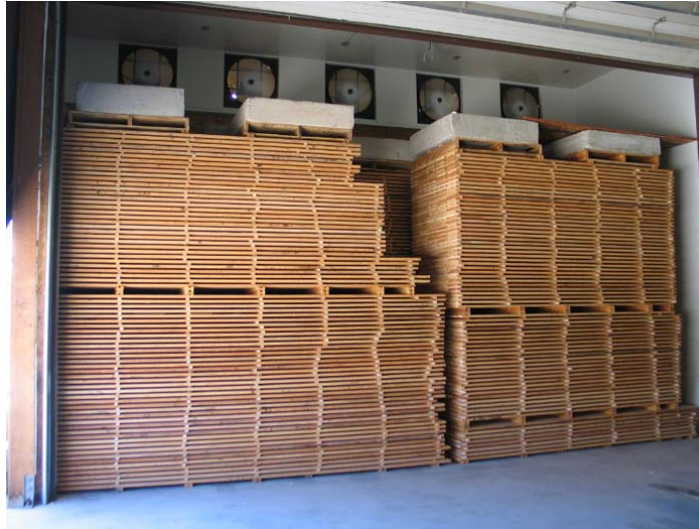
Figure 9: Example of Lumber Stacked in a Kiln. Notice the Small Pieces of Wood (Stickers) Vertically Aligned in Between Each Piece of Lumber.
