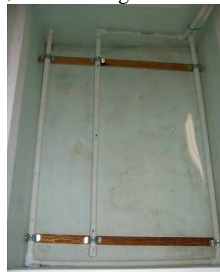
Interior of a standard 1,000 lb tote converted to a chiller tote by Doug Drum of Indian Valley Meats, at a cost of less than $50 for tubing and connectors.
