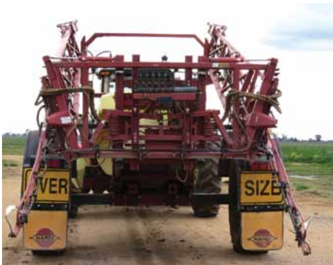
The boom spray was purchased so that the axle width could be easily modified to 3m wheel centres.
