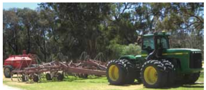
Hicks Farming use John Deere Greenstar™ RTK autosteer and John Deere GS2630 with dry rate controller into a Horwood Bagshaw electric drive airseeder for variable rate fertiliser application.
