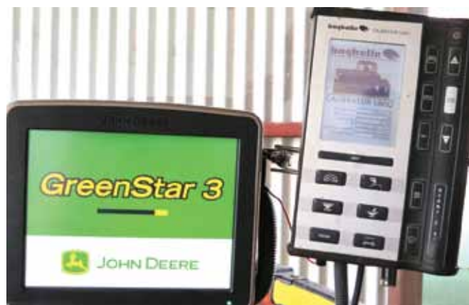
Compatibility of implement controllers is essential for PA and variable rate applications. The Bogballe spreader controller is easily operated with the John Deere system.
