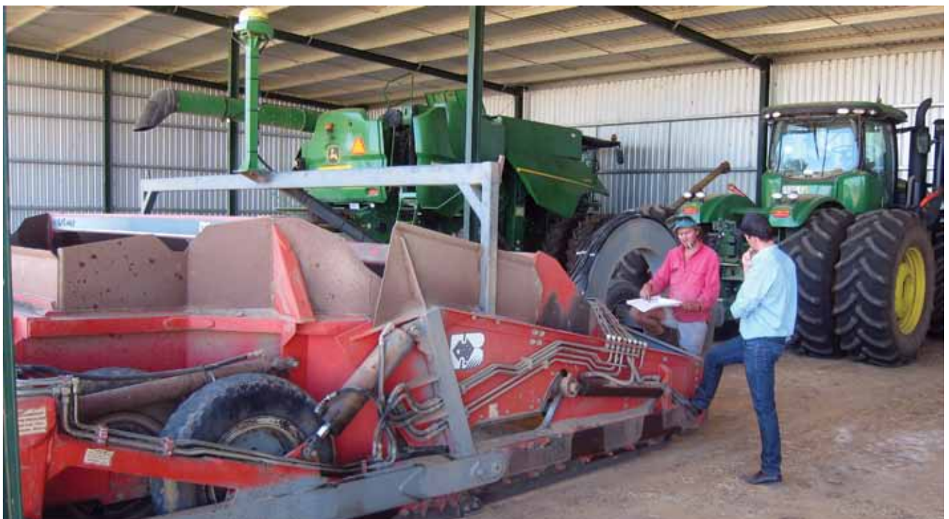
Arnold Farming had to invest in their own RTK base station to successfully use iGrade on their land-levelling bucket. The bucket has a receiver fitted to it so that accurate levels can be achieved.
