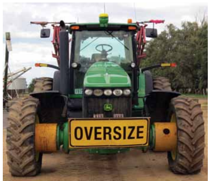
Cotton reels were fitted to the front axle and wheels spread on the rear axle of the tractors to move to 3m wheel centres for the CTF system.
