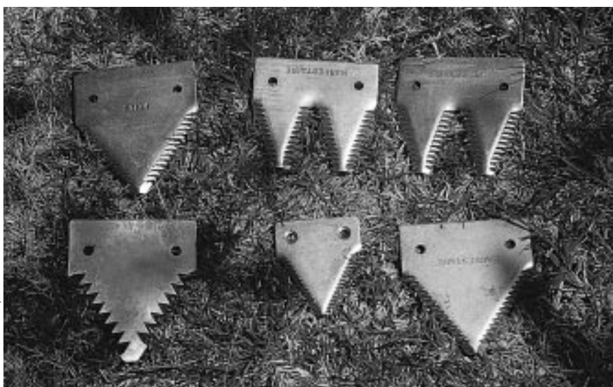
A range of cutterbar knives including double cut (top right) and more aggressive teethed standard sized knives. The smaller knife (middle bottom) is from a Massey Ferguson closed front.
