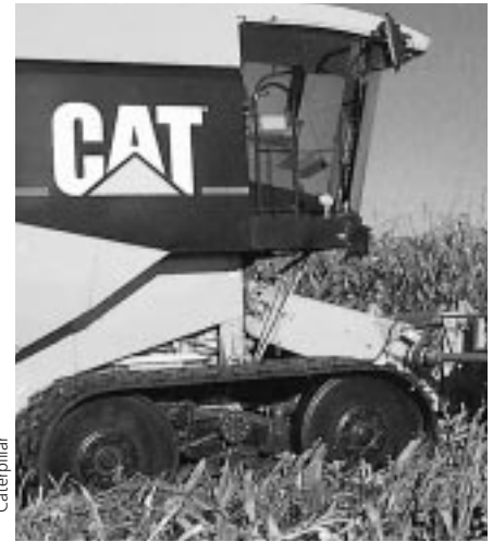
Three forms of ground drives for rice fields. High flotation tyres on front and rear -powered axle (left), half-track conversion (centre) and full-track as original equipment (right).
