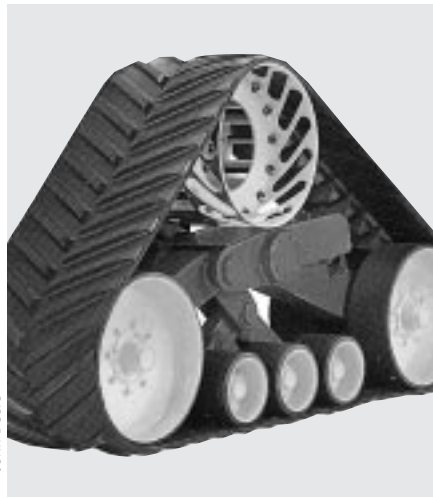
Three forms of ground drives for rice fields. High flotation tyres on front and rear -powered axle (left), half-track conversion (centre) and full-track as original equipment (right).
