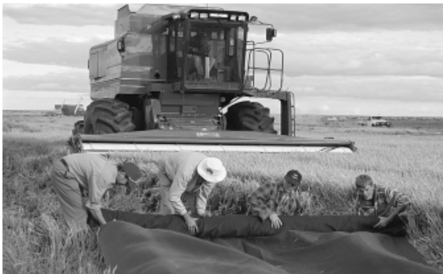
Kondinin Group researchers collecting material other than grain (MOG) after harvesting with a Case 2188 fitted with a Shelbourne Reynolds stripper front.
