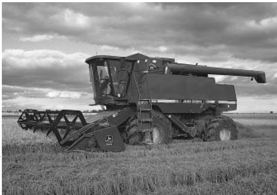
Conventional grain head showing pickup reel, cutterbar and auger.
