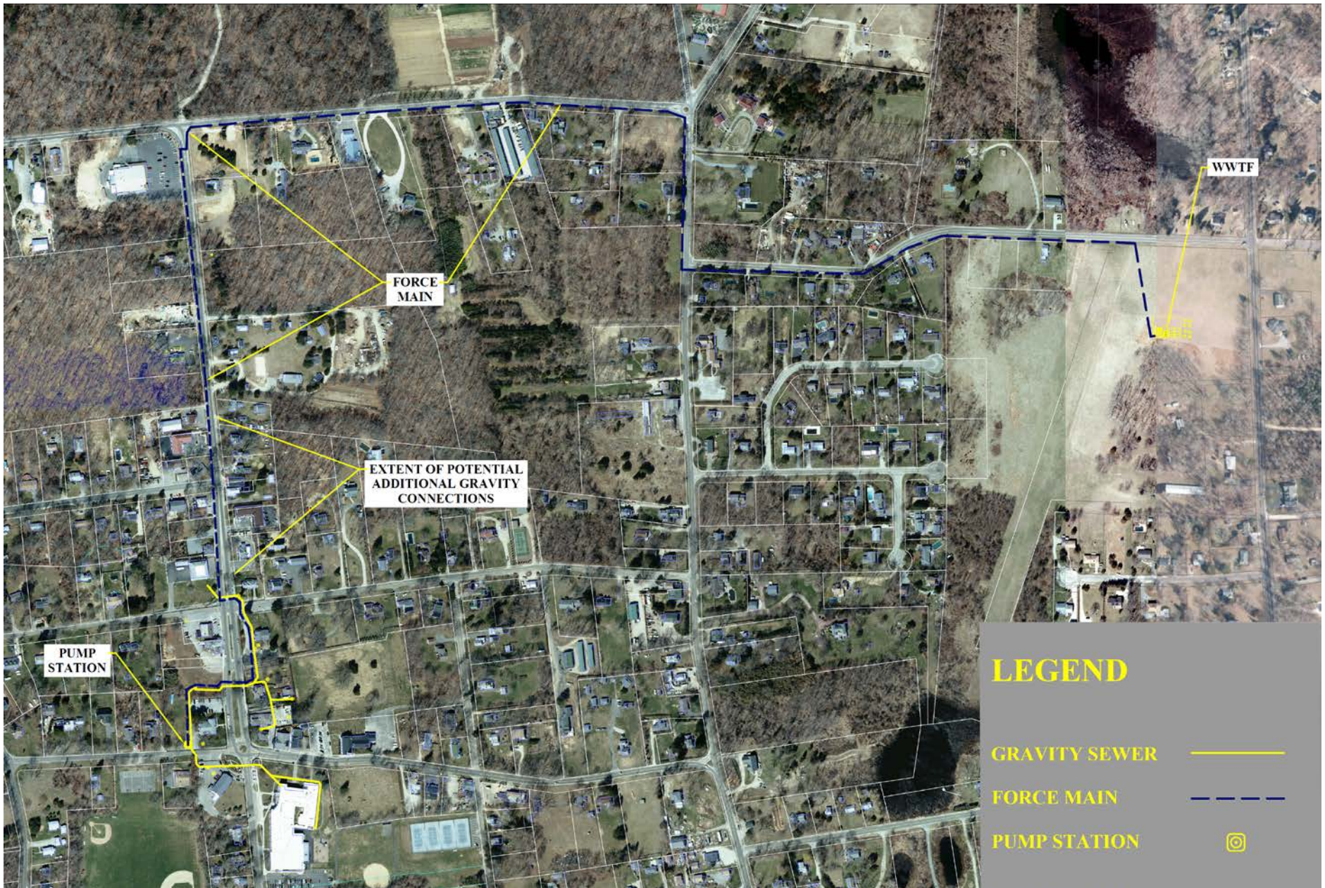
Figure 4-9 Preliminary Collection System Layout – Airfield Site
