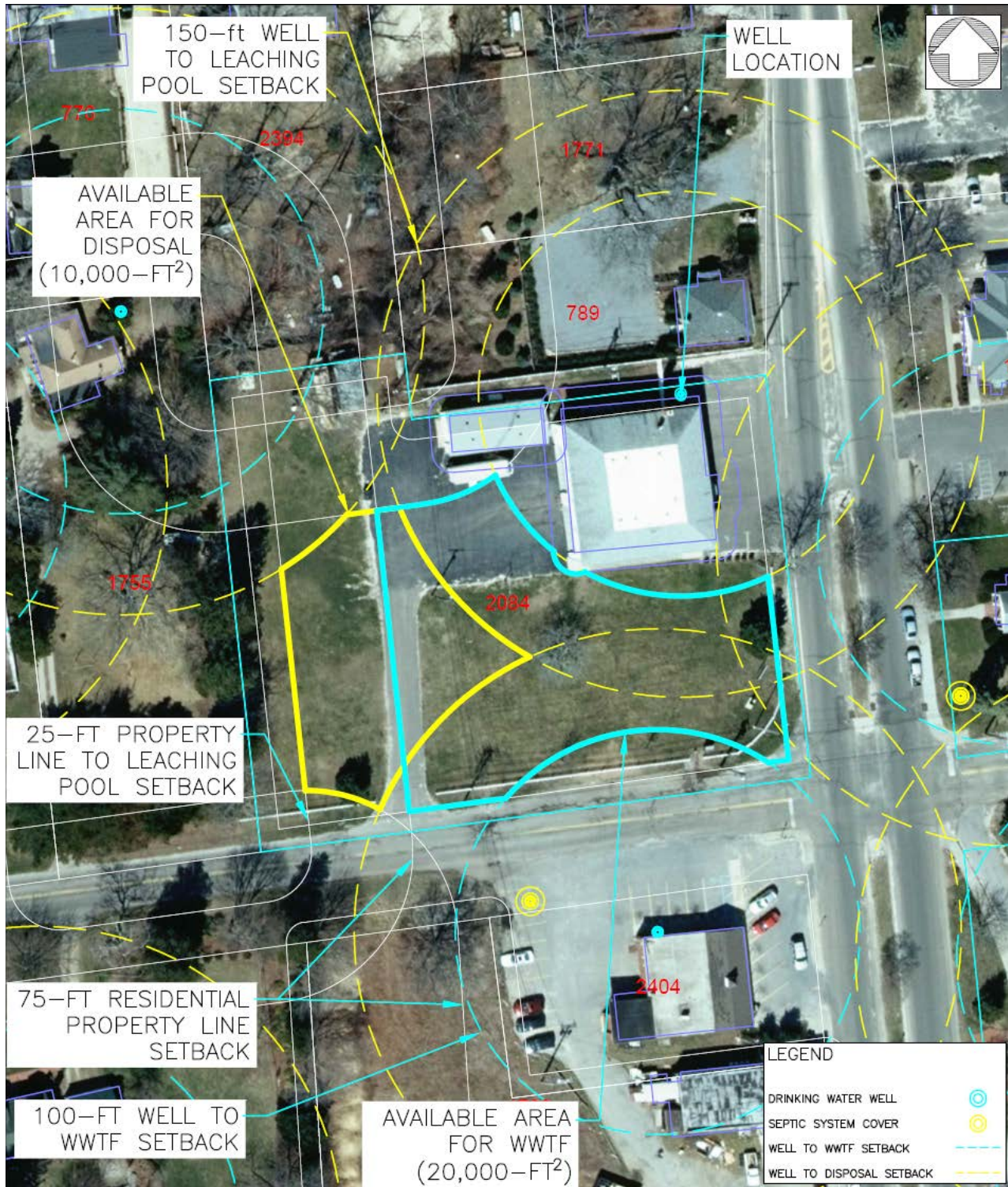
Figure 2-2 Fire Department Site Available Area Analysis
