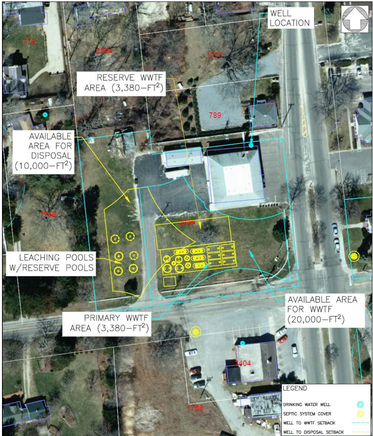
Figure 4-3 4,225-gpd Nitrex System Layout – Fire Department Site
