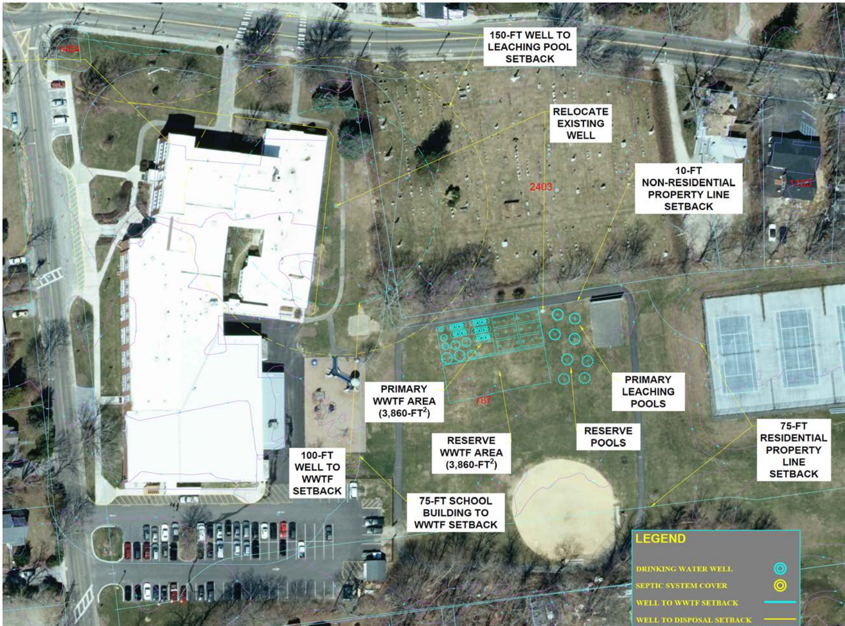
Figure 4-5 6,200-gpd Nitrex System Layout – School Ballfield Site
