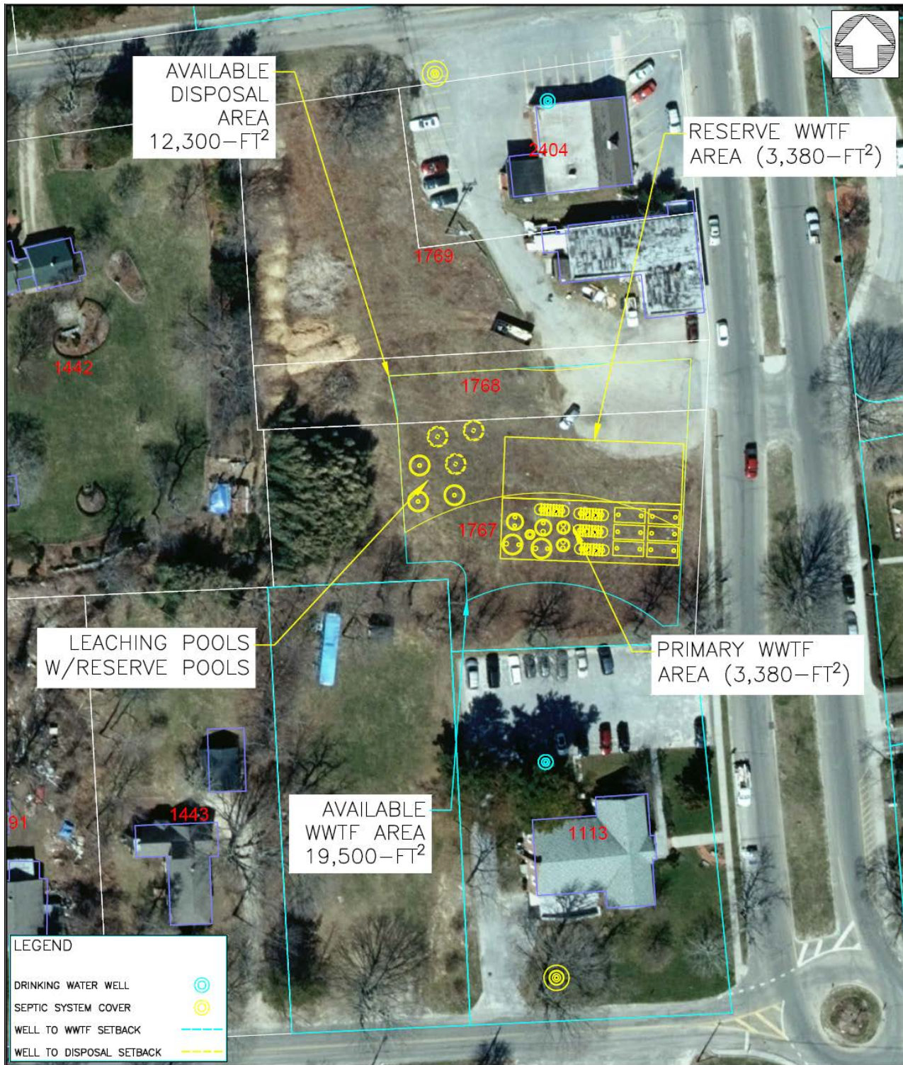
Figure 4-4 4,225-gpd Nitrex System Layout – Library North Site
