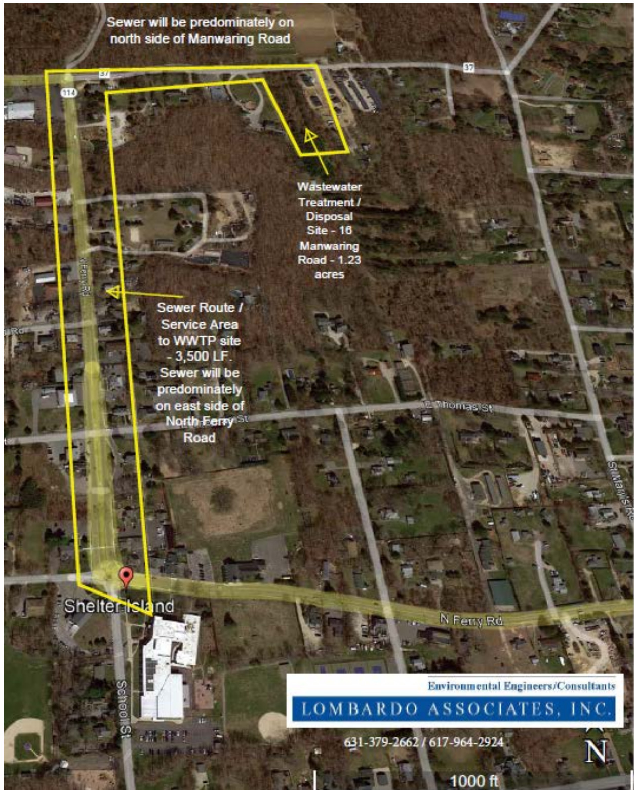
Figure 1-1 SI Municipal Wastewater System Layout
