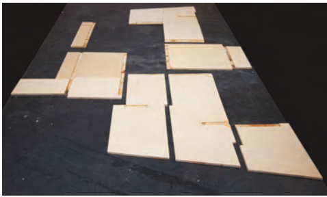
Jigsaw house model wall panels prior to assembly. Solid timber floors interlock into walls.
