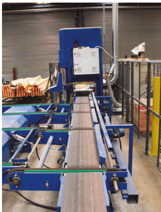
CNC machinery cutting timber for frames and trusses, at PlaceMakers.
