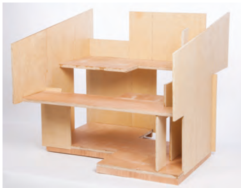
Jigsaw house assembly. Note interconnected floors and walls.
