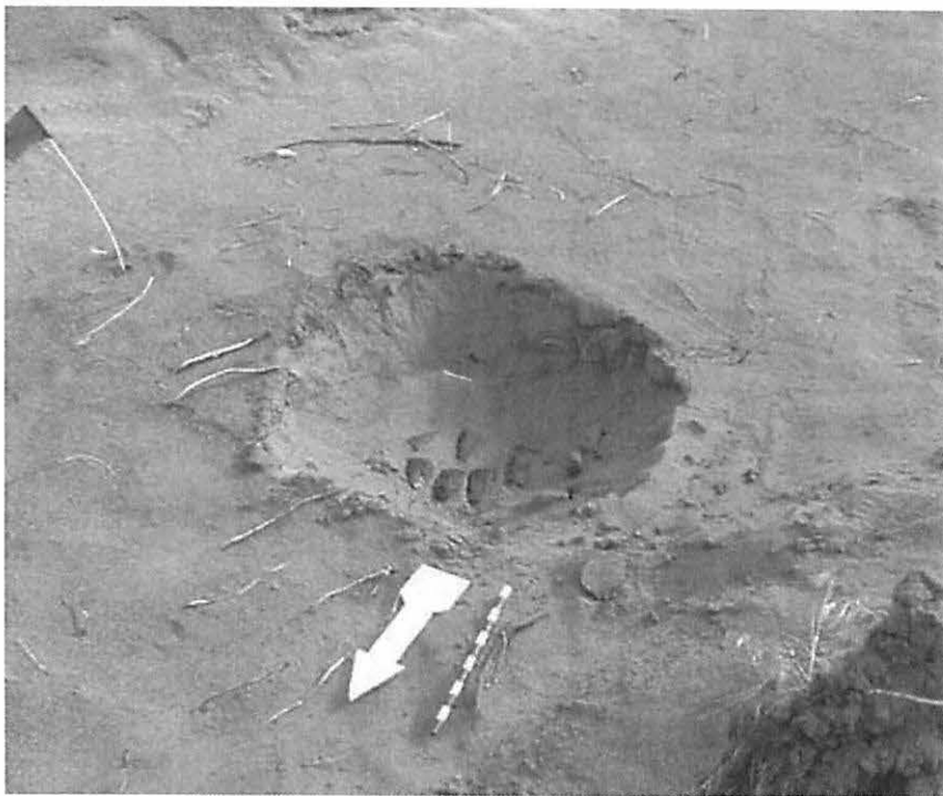
Fig. 10. Photograph showing the simulated cache of lithic materials, constructed at the 24 in. depth level of the Remote Target Test Bed. These small artifacts reflected no radar energy due to their small size.
