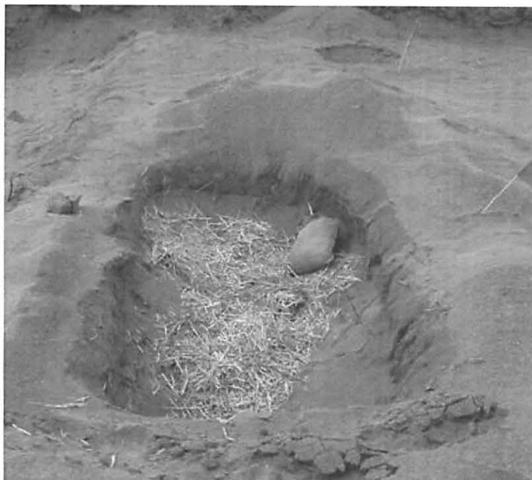
Fig. 11. Photograph showing one of three simulated human burials, constructed in the shallow level of the Remote Target Test Bed using organic material. These features produced no reflections because there is not a distinct surface from which to reflect radar energy.
