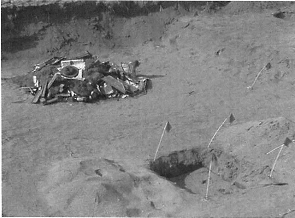
Fig. 9. Photograph showing the simulated trash pile and un-burned earth oven (in the foreground), constructed in the medium depth level of the Remote Target Test Bed. The trash pile contains many metal objects that reflect radar energy, but the earth oven was un-fired and therefore did not have a surface from which to reflect energy.
