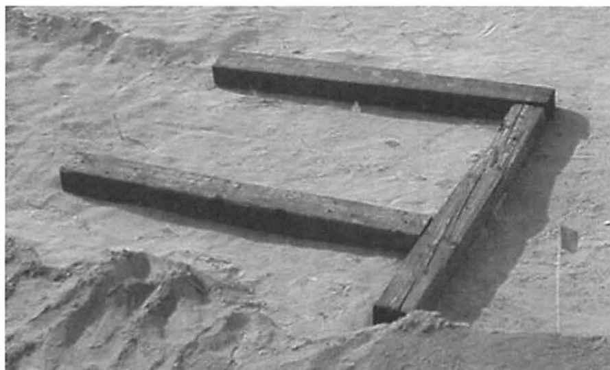
Fig. 12. Photograph showing the railroad ties placed at the deepest portion of the Remote Target Test Bed. The railroad tie feature produced no reflections when the ground was dry. When the ground had been saturated with water and then left to drain for 2 days, these ties retained water like a porous sponge, while the water drained readily from the surrounding sand. As expected, the saturated railroad ties reflected radar waves.
