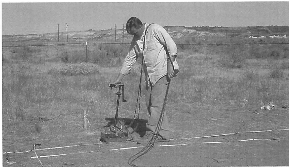
Fig. 4. Photograph of technician collecting GPR reflection data at the Remote Target Test Bed, using a Sensors and Software 450 MHz antenna.
