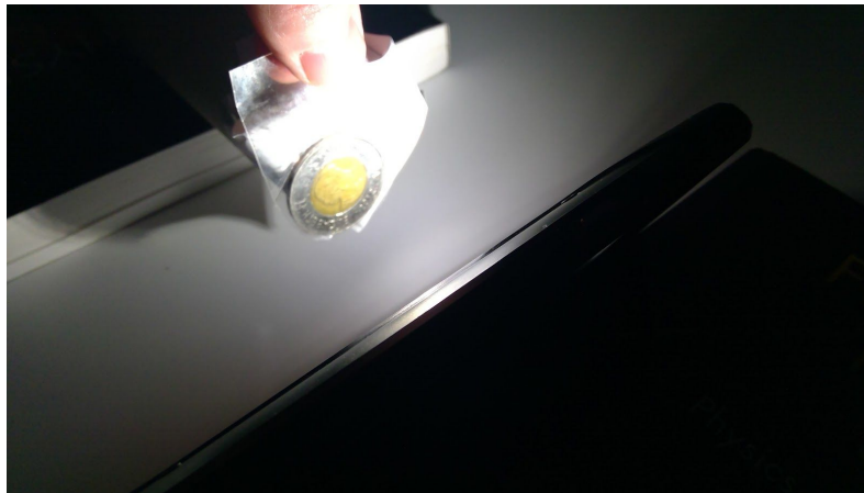
Figure 16: It is best to have the coin very close to the paper, to make sure the shadow is smaller than the hole.
