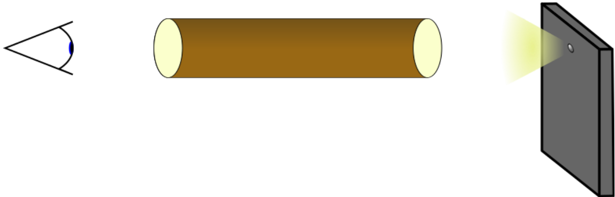
Figure 14: The flashlight shines into one side, and the observer looks at the other
