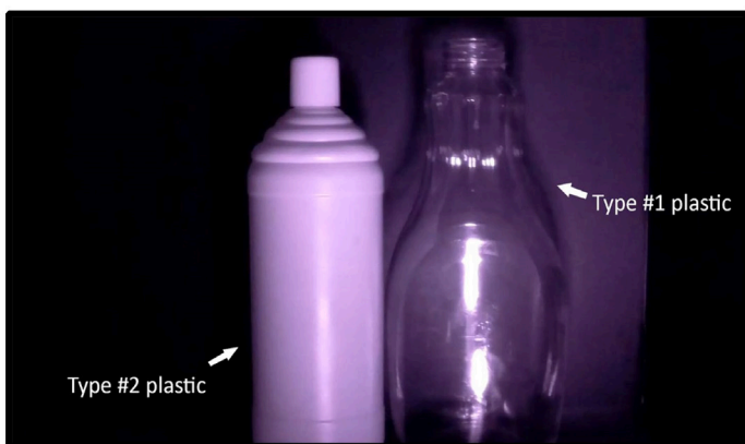
Figure 5: Types #1 and 2 plastic bottles with NIR light at 850 nm.
