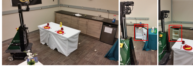
Fig. 7 Robot performing Case study 1. (a) scanning environment, (b) looking for bowl in refrigerator, (c) looking for and finding bowl in cabinet.
