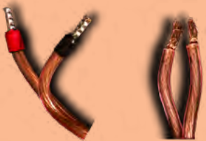
Fig. 2: Exposed ends of the speaker wire. L: Crimped, R: Uncrimped.
