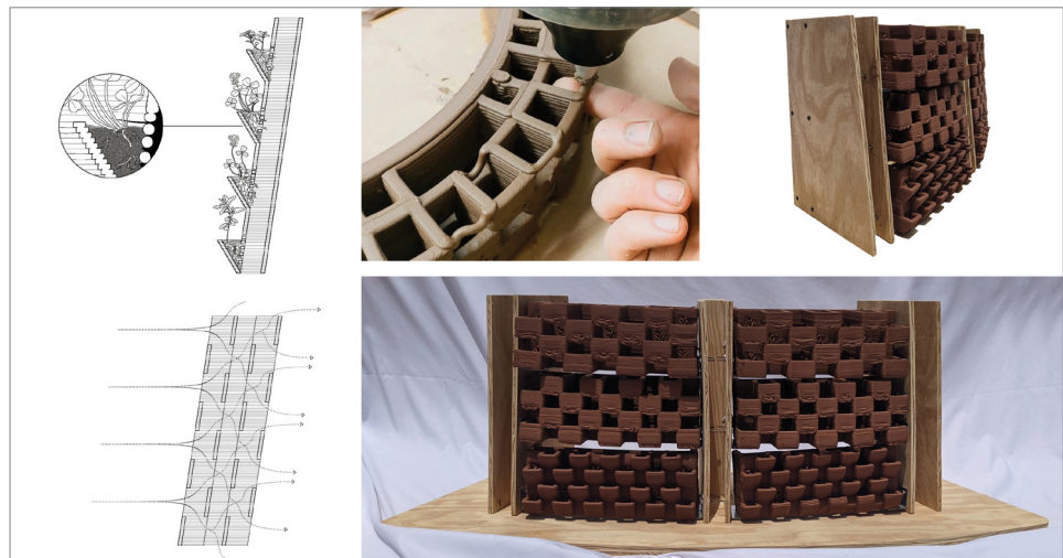
Figure 5. Vertical Understory (B. Cornett and K. Macumber). Stackable modules integrate pockets and apertures that allow for plant habitats and natural ventilation (left). The printing process requires temporary support of the cantilevers (top center), producing a range of pocket types in the full-scale mockup (bottom and top right).
