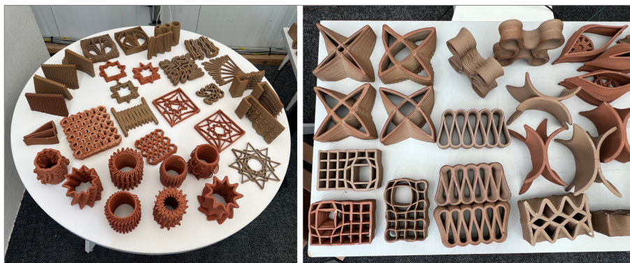
Figure 1. Initial 3d printed ceramic material studies and prototypes testing different techniques for toolpath design, texture, aperture, and modulation
