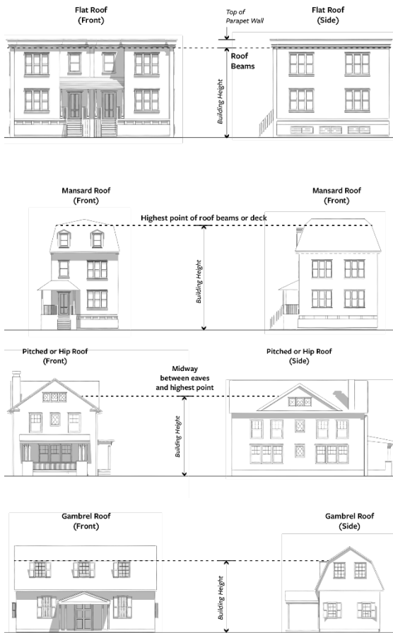
FIGURE 7-E: BUILDING HEIGHT MEASUREMENT
