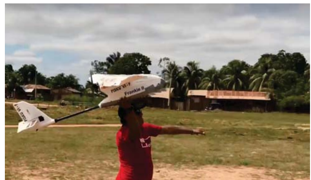
Fig. 2. The Event 38 E384 fixed-wing drone, as operated by WeRobotics, being hand-launched in Pucallpa, Peru (image from [25]).
