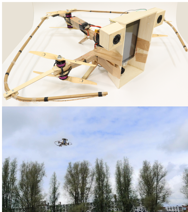
Fig. 1. Top: The prototype wooden-frame drone was developed for use in Denmark to assist in land-based search and rescue operations. The frame - comprised of a mahogany and balsa sandwich structure - exhibited high stiffness and low weight. Bottom: The final drone was able to withstand outdoor testing (upper photo by the authors; lower photo by Andreas Aagaard Asmussen and Nikolaj Pihl Thomsen).
