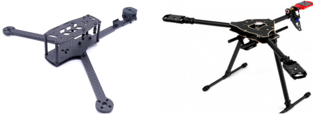
Fig. 4. Two examples of commercial Y-copter drone frames [12][13]. The fiber patterns reveals the fiber directions - at least of the outermost layers. Two typical construction approaches are shown: arms made of flat plates with 0/90 degree fibers (left), and arms made of hollow tubes, also with 0/90 degree fibers (right).
