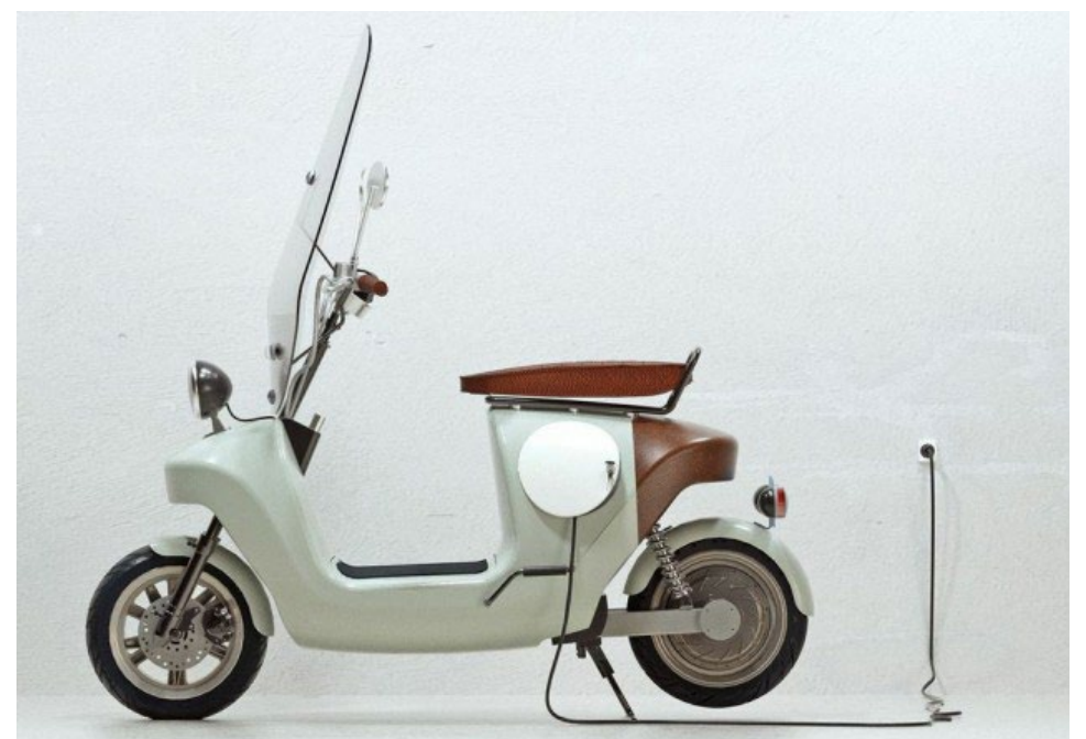
The Be.e electric scooter is made of 90% hemp fibre, 10% flax fibre and glue. Designed by Waarmakers for Van.Eko http://www.vaneko.com/the-be-e/
