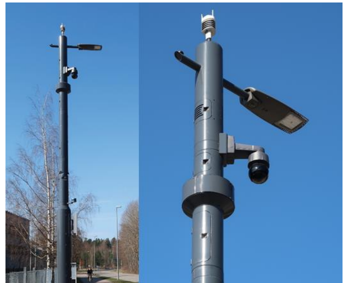
Figure 5. Real-life smart pole prototype in Kera, Espoo, Finland with lighting, weather, traffic monitoring, camera, public announcement, surveillance and LIDAR modules.
