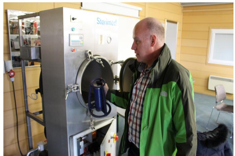
Sterilization expert Joost van Doornmalen performing tests with the 3M Electronic Test System (ETS). ©Andreas Larsson/MSF
