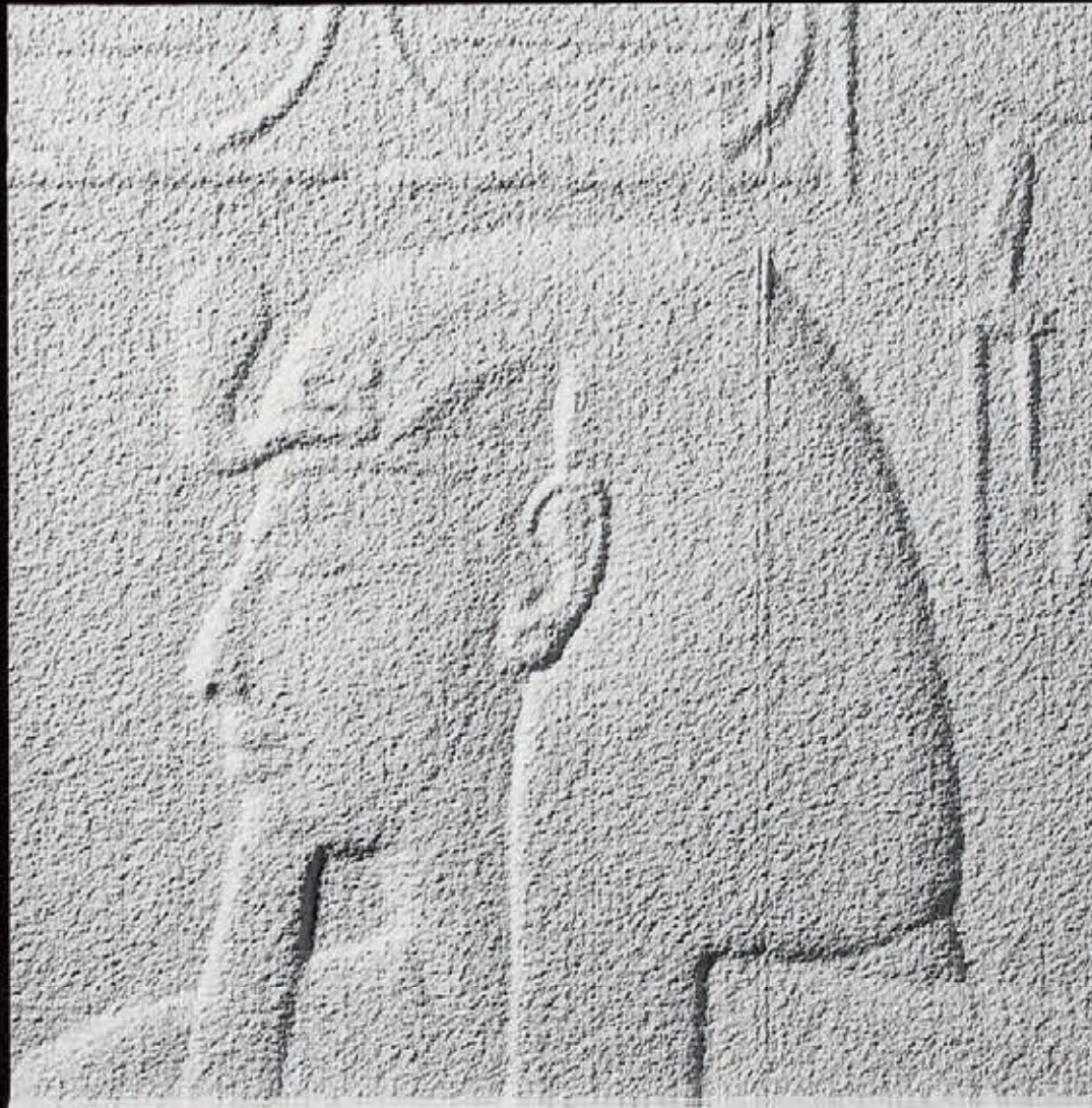
Faro Focus 3d X130 used at close range at maximum resolution Tomb of Seti I (detail) Recorded from 1.4 meters
