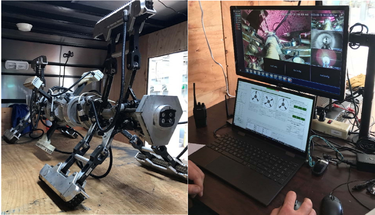
Figure 3: MOCCASIN ILI Tool Configured for 30in PIPE & Control System
