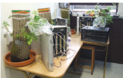
Air entrainment capturing volatile emissions from leaves on Oak logs in the laboratory 2016
