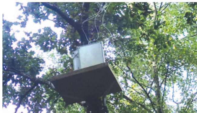
Air entrainment equipment for identifying volatiles for beetle trapping placed high up in tree crowns in the Forest of Dean
