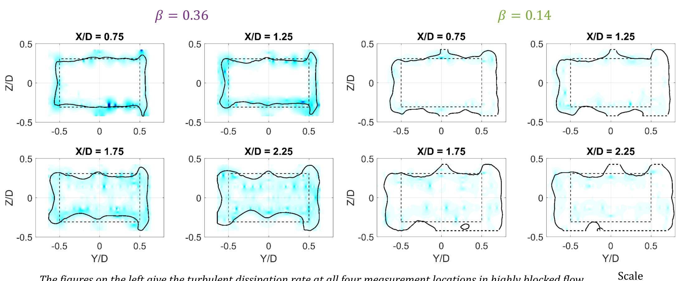
The figures on the left give the turbulent dissipation rate at all four measurement locations in highly blocked flow. The analogous figures on the right indicate that the dissipation rate is lower at a lower blockage ratio. This is to be expected, given the larger difference between the wake and bypass flow at higher blockage, which results in more shear and causes additional energy to be dissipated downstream.
