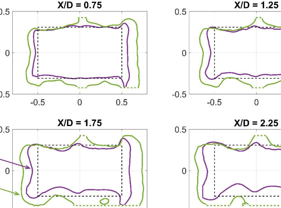
Solid lines denote the boundary between the wake and bypass flow. The wake tends to narrow as blockage increases.
