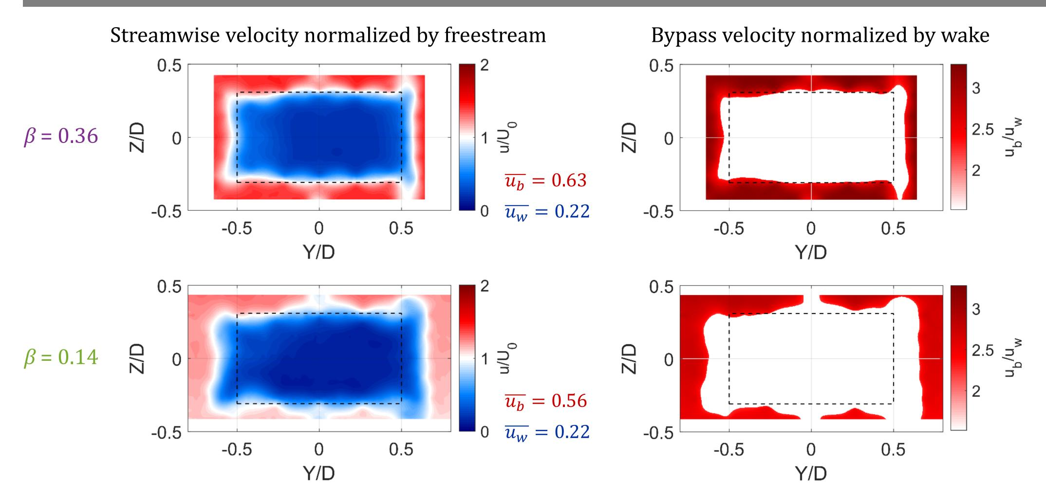
The figures on the left indicate that the bypass velocity increases as the blockage ratio increases. However, the wake velocity remains relatively unchanged. This causes a larger difference between the two flows at higher blockage, as shown by the figures on the right.
