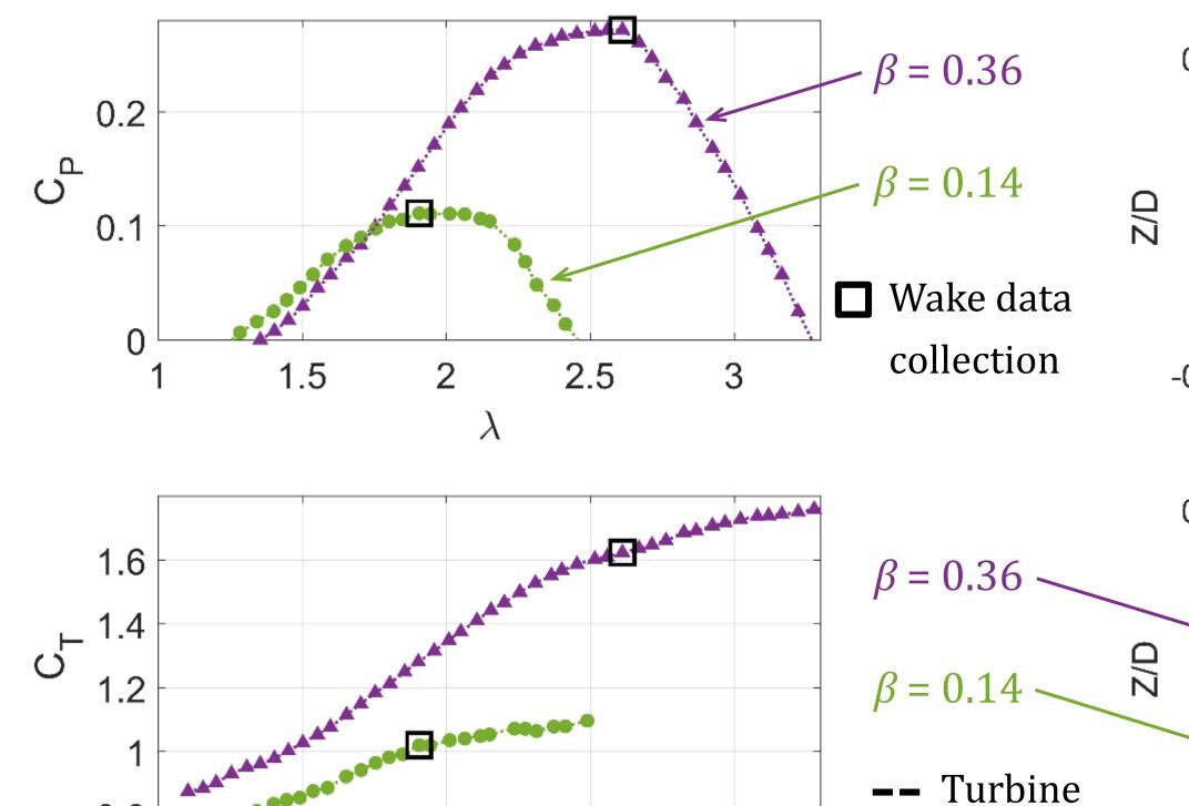
Blockage increases a turbine's power and thrust coefficients. Wake data were collected at the highlighted tip-speed ratios.
