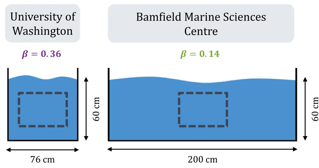
Tests were conducted at varying blockage ratios ( $\beta = A_{turbine}/A_{channel}$ ). The water temperature, inflow speed, and channel depth were fixed to achieve constant Reynolds and Froude numbers between tests.
