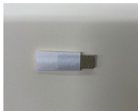
Figure 4d: Close-up of a paper pocket housing a magnet. Image by Yuhong Zhang.
