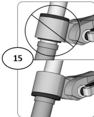
Insert the hitch around the bushing. Drop the receiver onto the hitch, then insert and secure the quick release pin.
