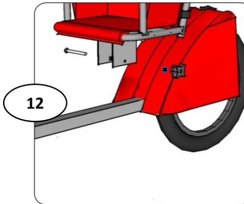
You may also use pliers on the knob to help tighten. Continue tightening until there is little to no movement on the frame.
