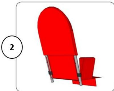
Install the arm rests to the seat base. Insert the armrests through the fabric sleeves. Secure the hook and loop closure.
