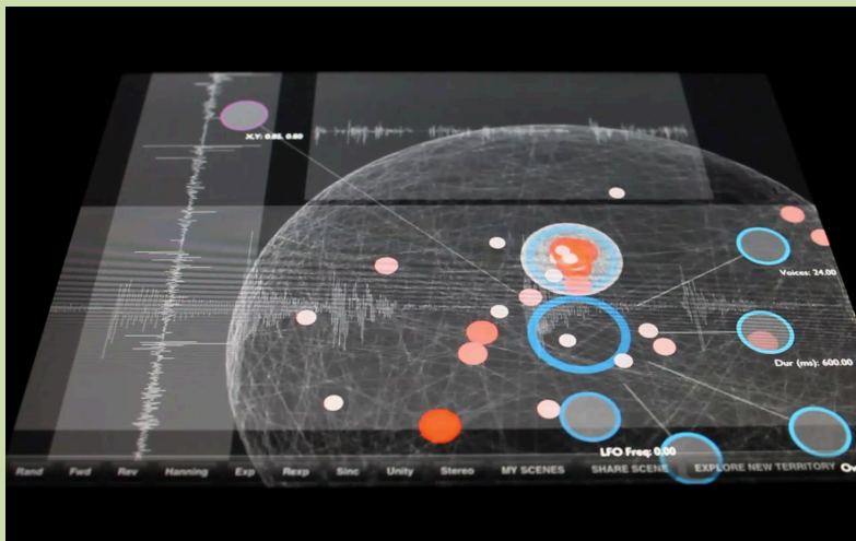
Figure 6. Borderlands app for iPad. The user slides (“scrubs”) a circle along the waveform to select segments to granulate. The attached satellite circles function as potentiometers controlling granular synthesis parameters. Another recent scrubbing app is MegaCurtis.
