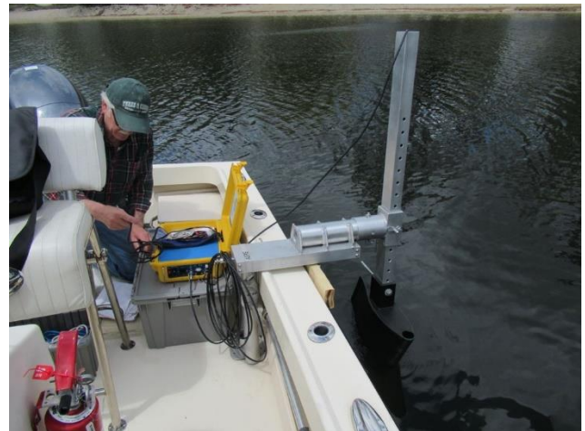
Hilary Snook (US EPA) setting up a sonar transducer and recording computer to assess dominant bottom substrates in Georges Pond on June 5, 2018. (Photo: Brian Friedmann, GPA)
