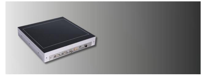
The 2824HR is a dynamic X-ray detector designed specifically for industrial NDT, pathology and other CT applications such as X-ray diffraction, with a pixel pitch of 50 µm and high-resolution Csl or Gadox scintillator. This detector employs a state-of-the-art high-resolution CMOS sensor with 14-bit digital outputs and two gain modes offering a high dynamic mode or a high sensitivity mode ideal for low dose, real-time imaging.
