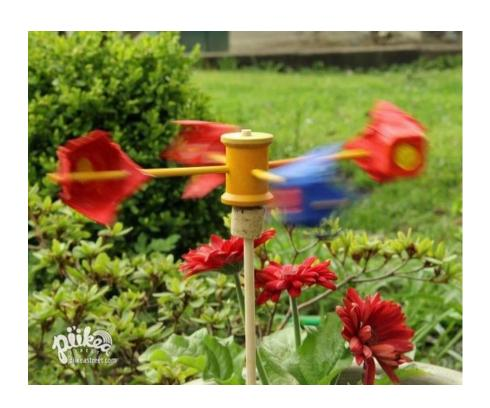
Build a DIY anemometer. To measure wind speed.
