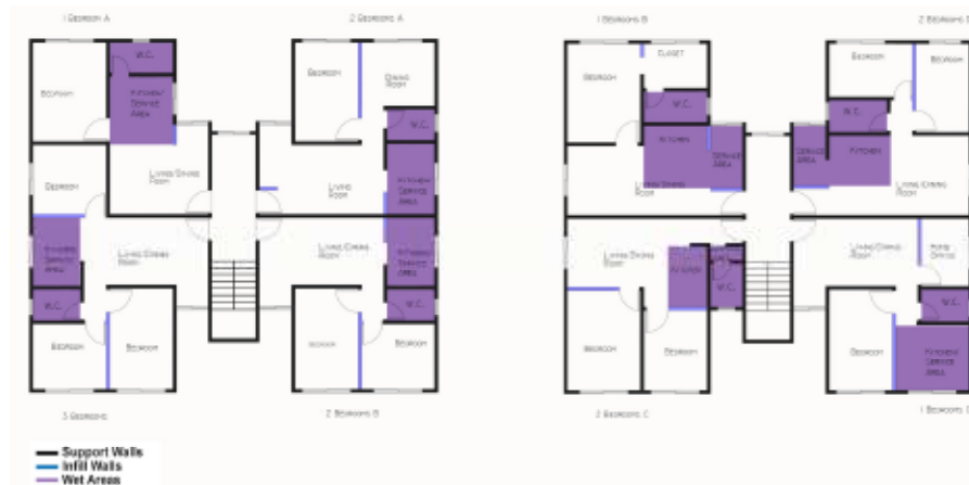
Figure 5- Floor-type of the Residencial Monterrey I with adequation to the OB. Source: (Authors 2018)
