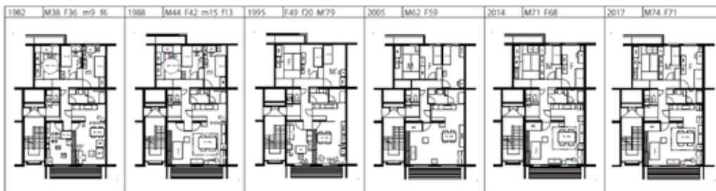
Figure 2: An example of layout changes and renovation of a unit in the apartment Source: (Author 2018)
