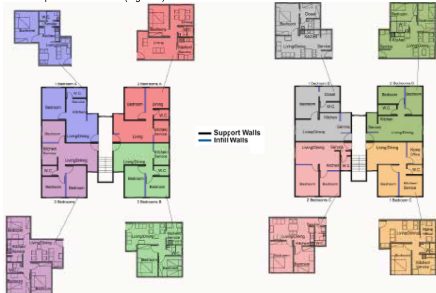
Figure 7- New possibilities of layout from the adjustment of the system. Source: (Authors 2018)
