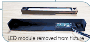
LED module removed from fixture
