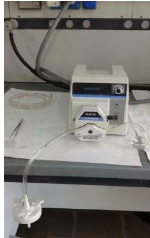
Figure 18. Peristaltic pump used for filtration.
