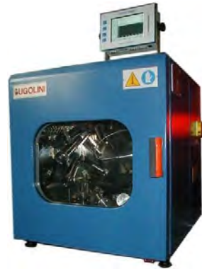
Figure 21. Laboratory exhaustion machine (Source: Ugolini)
