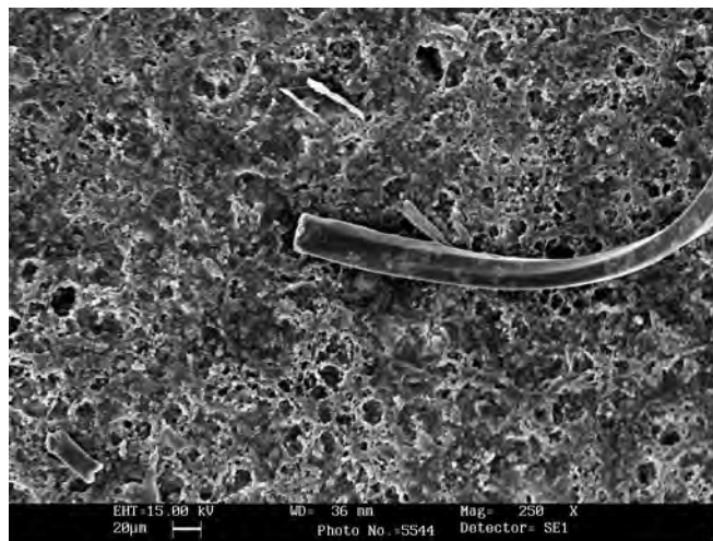
Figure 44. Fiber released by raw white textured polyester sample (PES#1).
