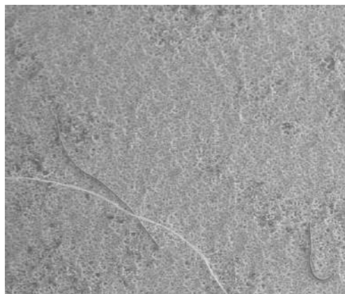
Figure 34. Magnification of a SEM micrograph showing a cotton fibre (white)
