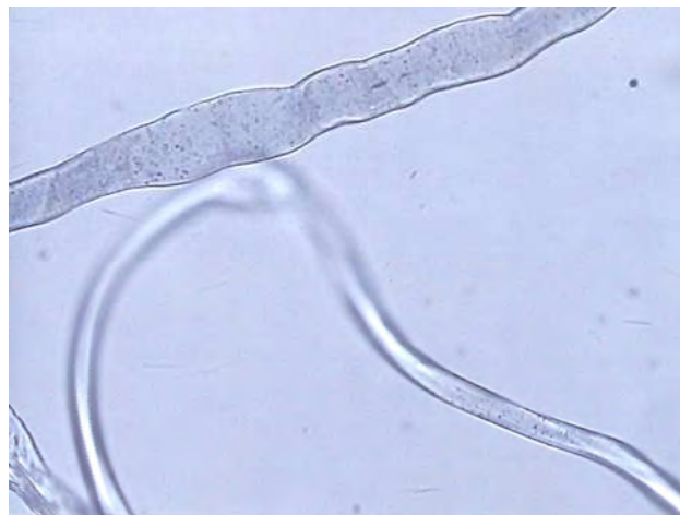
Figure 31. Light microscopy image of polyamide found in the filtration residue.
