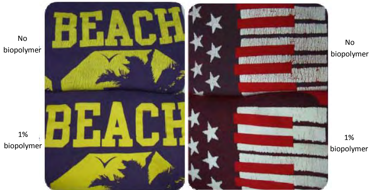
Figure 26. Printed t-shirts washed 10 times with and without using a biopolymer as additive (Source: Croda)
