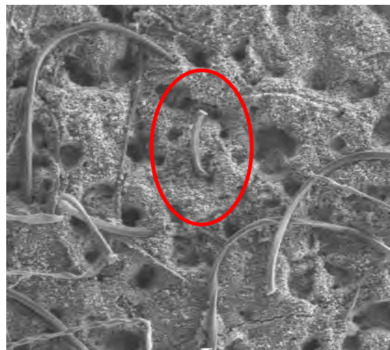
Figure 35. SEM micrograph of a magnification of a filter containing fibres coming from a knitted polyester textile (PEP) washed with Detergent Powder 1 (DP1)
