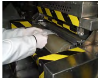
Figure 20. Laboratory padding machine (Source: LEITAT)
