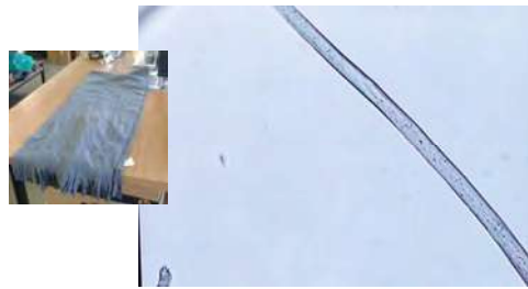
Figure 24. Light Microscopy photos of fibers from 100% polyester scarf; 200X.
