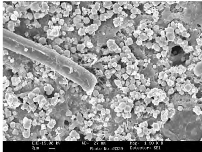
Figure 38. SEM image of polyester fiber on filter.
