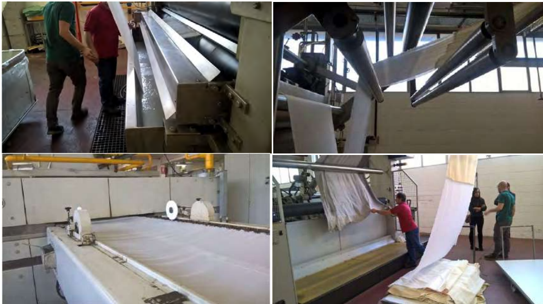
Figure 27. Impregnation, padding, drying and curing process in the industry.
