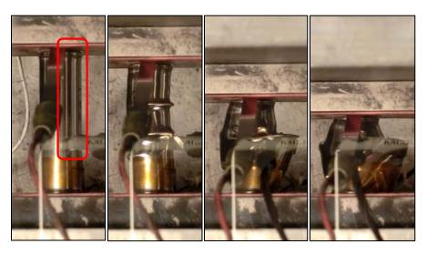
Figure 1: Cylindrical lithium-ion cell undergoing axial crush between two flat plates
