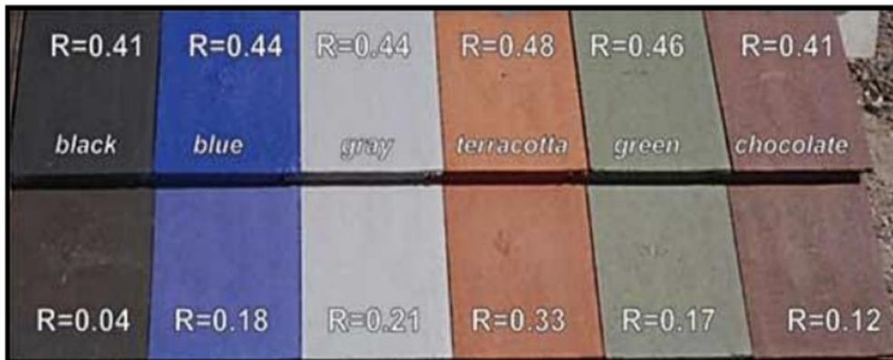
Figure 9.1. Cool-colored tiles (top row) look like conventional roof tiles (bottom row) but have higher solar reflectance. 174
