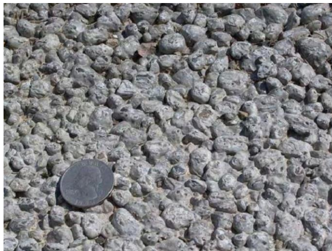
Figure 9.37. Example of pervious concrete pavement surface layer, with quarter to for scale. 405
