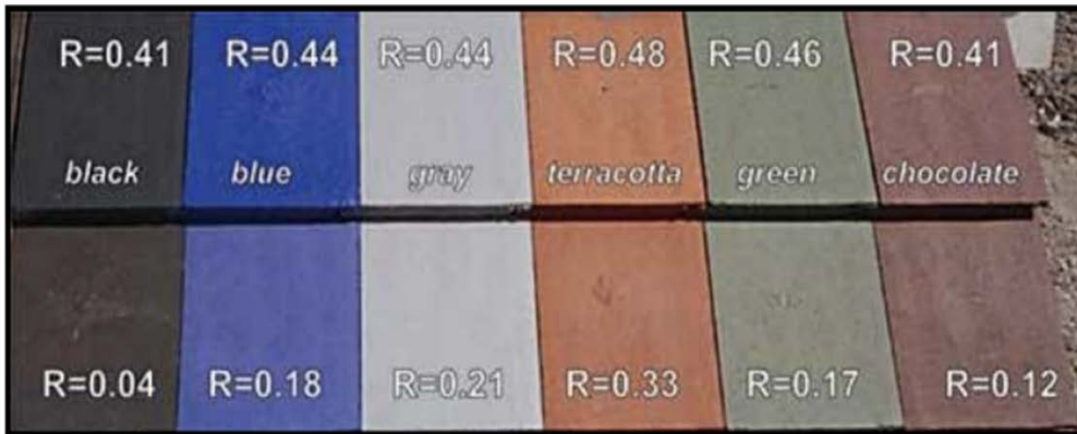
Figure 9.1. Cool-colored tiles (top row) look like conventional roof tiles (bottom row) but have higher solar reflectance. 173
