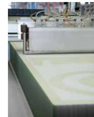
4 Impression. Les buses déposent un liant aux endroits définis. Printing. Nozzles project bonding agent at precise points as programmed.
