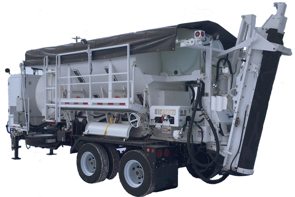
Figure 4: Volucon-ProAll specialised runway repair volumetric mixer
