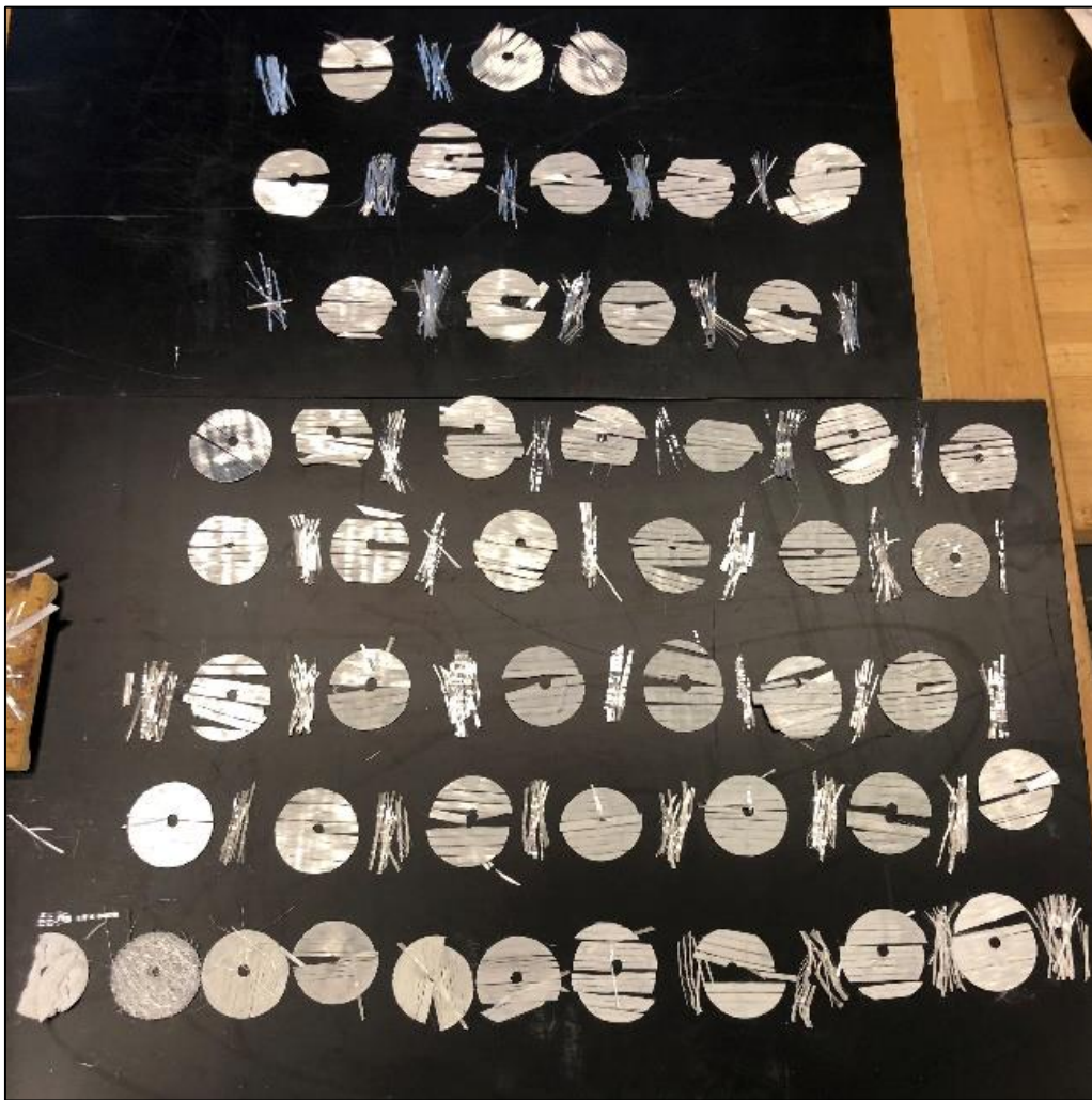
Figure 5. Fiber layout verified from ASTM D2584 burnout test of a spar cap sample from Station 7.
