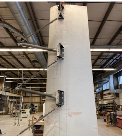
Figure 14: UC and Braced Line Post hardware is completely installed and blade is erected in the lab awaiting a full-scale structural test
