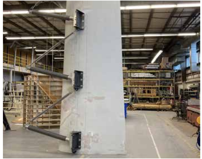
BladePole mock-up in laboratory
