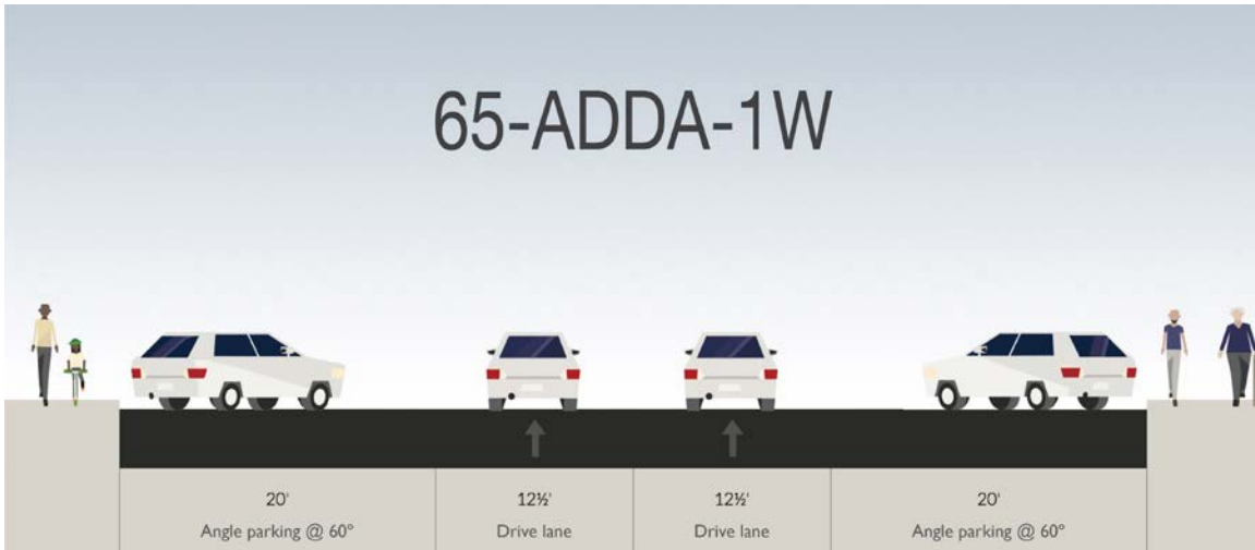
This cross section is recommended for 4 th Street between Civic Center Drive and Denver Avenue, viewed here looking east.
