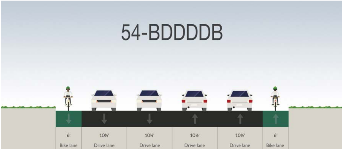
This cross section is recommended for Heavy Traffic Way between 3 rd Street and Houston Avenue.
