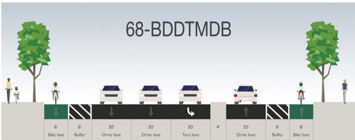
This cross section is recommended for 7 th Street between the IDL and 6 th Street, viewed here looking east.
