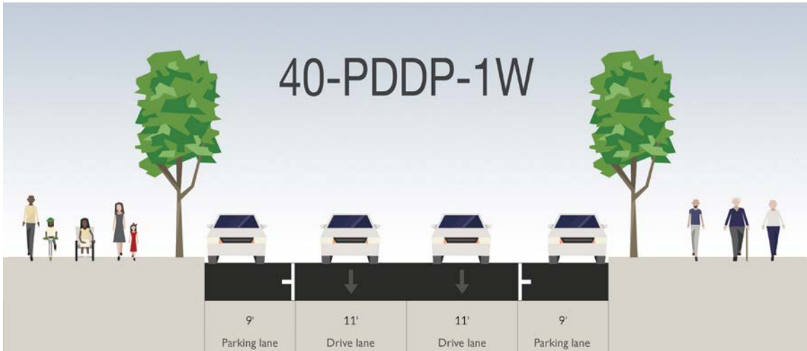
This cross section is recommended for 1 st Street between Greenwood and Hartford Avenues, viewed here looking east.
