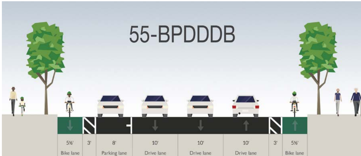
This cross section is recommended for Archer Street between Guthrie and Elwood Avenues, viewed here looking west.
