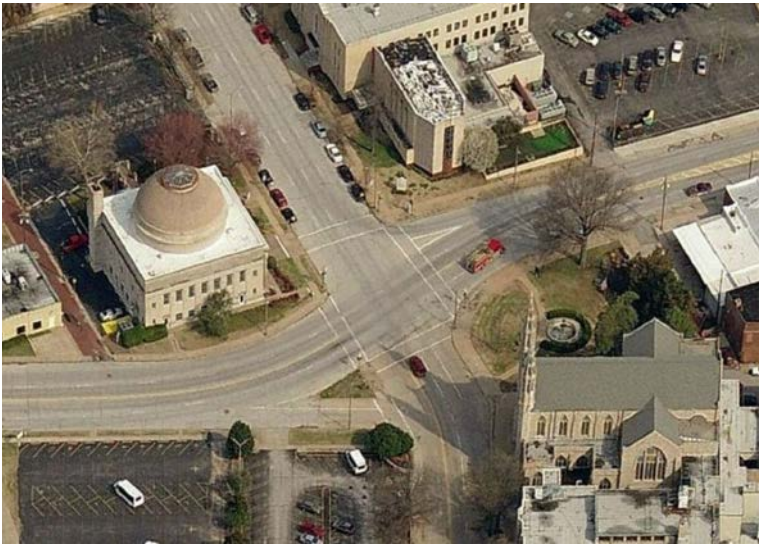
Route 66 was improperly allowed to swoop through downtown Tulsa with high-speed geometrics that make Cathedral Square unwelcoming to pedestrians.
