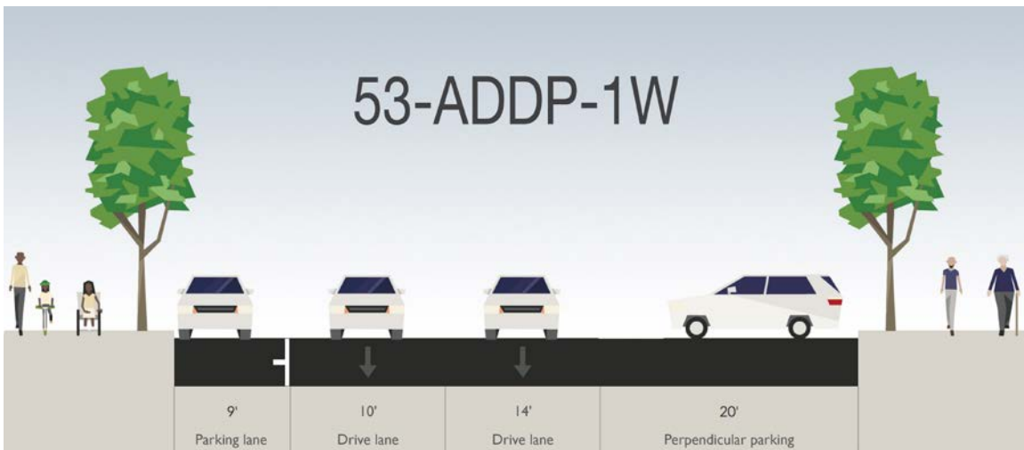
This cross section is recommended for 4 th Street between Frisco Avenue and Civic Center Drive, viewed here looking east.
