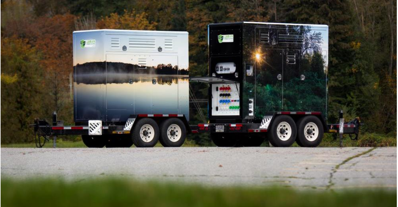
Designed specifically for entertainment production, MBSE Canada's Urban Power Source provides silent, zero-emissions power, replacing the need for diesel generators while filming on location. Photo credit: MBSE Canada
