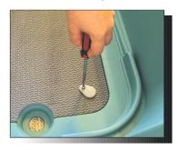
**2.** Attach plastic bolt caps using small Philip screws.
