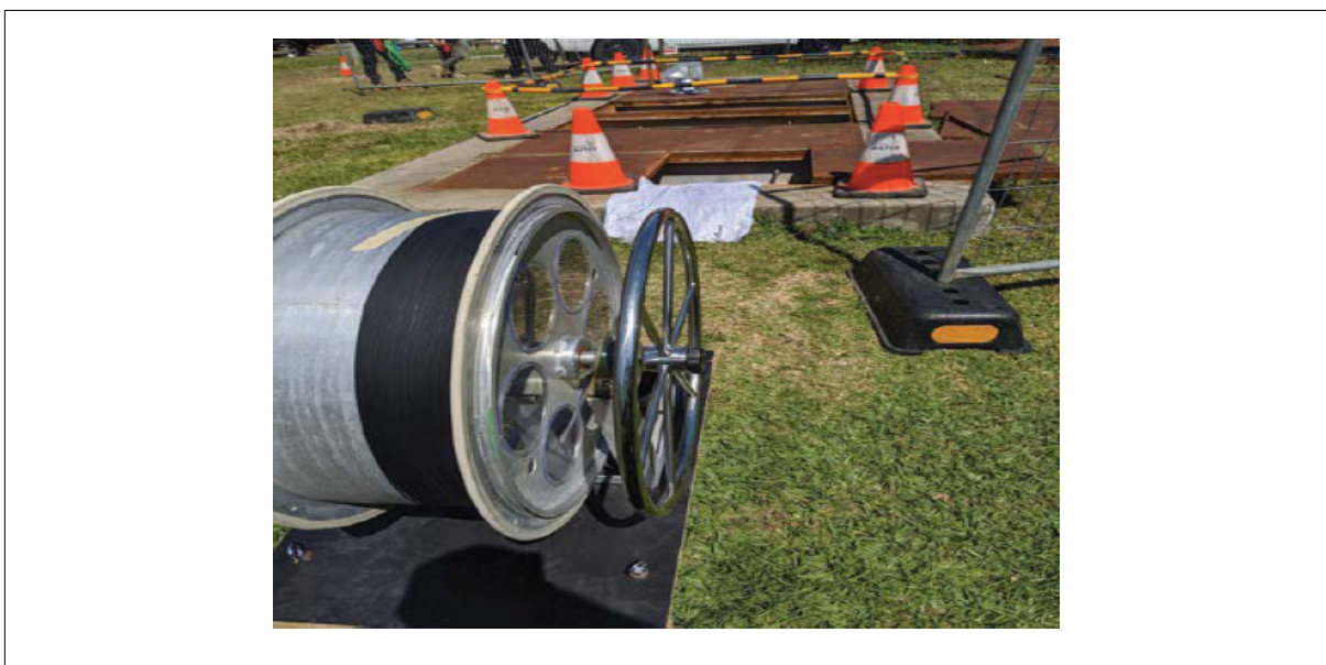
Figure 3.2: Tow cable and array off drum and into pipe through gap in plates. Drum and inboard system were placed on ground outside pit for duration of trial.
