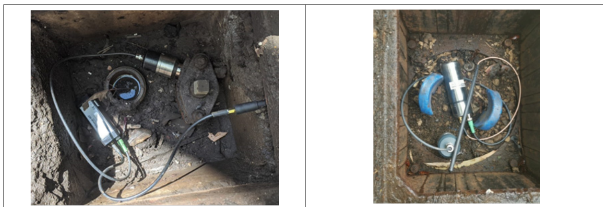
Figure 4.6: Von Roll Ortomat loggers: Sydney CBD (left), Bankstown (right).
