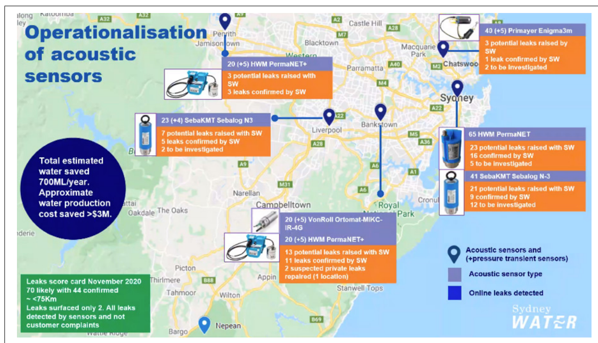
Figure 8.2: Location and types of acoustic sensors deployed across Sydney.
