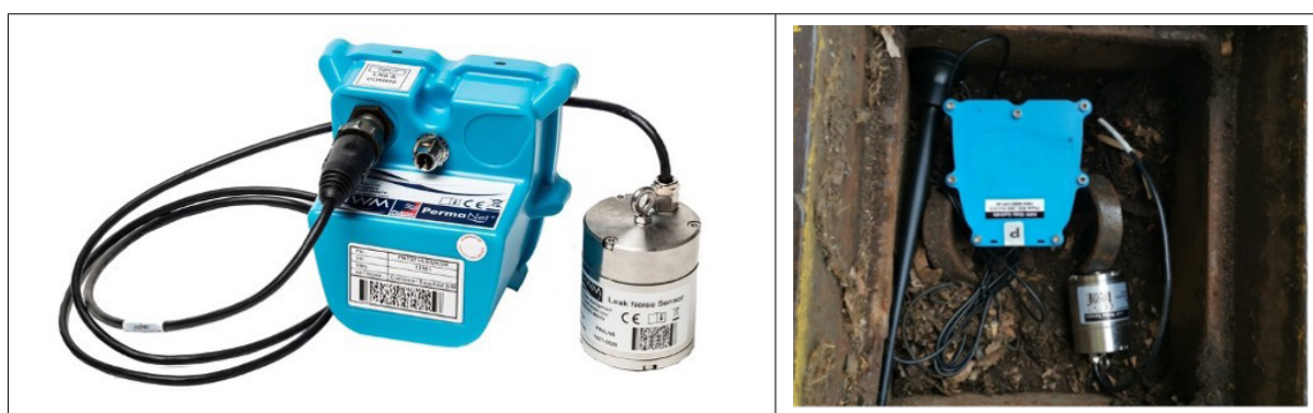
Figure 4.17: HWM PermaNET+ Logger and leak noise sensor. The left side image is as deployed.
