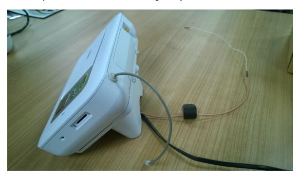
Extend the 312MHz antenna out from the rear of the unit. This will help to maximise the reception range of the sensor gateway at 312MHz.
