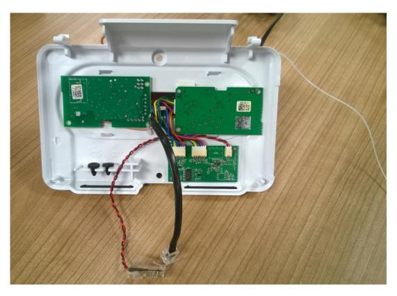
Step 3. Plug the mains adaptor into the Smart Hub socket labelled DC. Plug the twisted red and black cable into the socket labelled with a capital T. Then connect the adaptor to the mains power.
