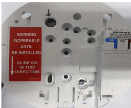
Fig 2: Showing the wiring to the Brooks smoke detector terminal block.
