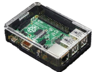
The Raspberry Pi 3 is powered by a +5.1V micro USB supply. Exactly how much current (mA) the Raspberry Pi requires is dependent on what you connect to it.
