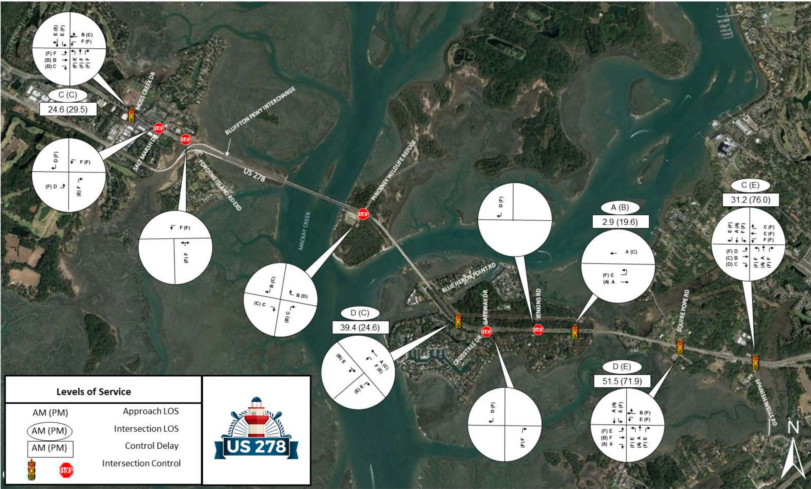
Figure 66: 2045 Reasonable Alternative 3 Intersection Levels of Service
