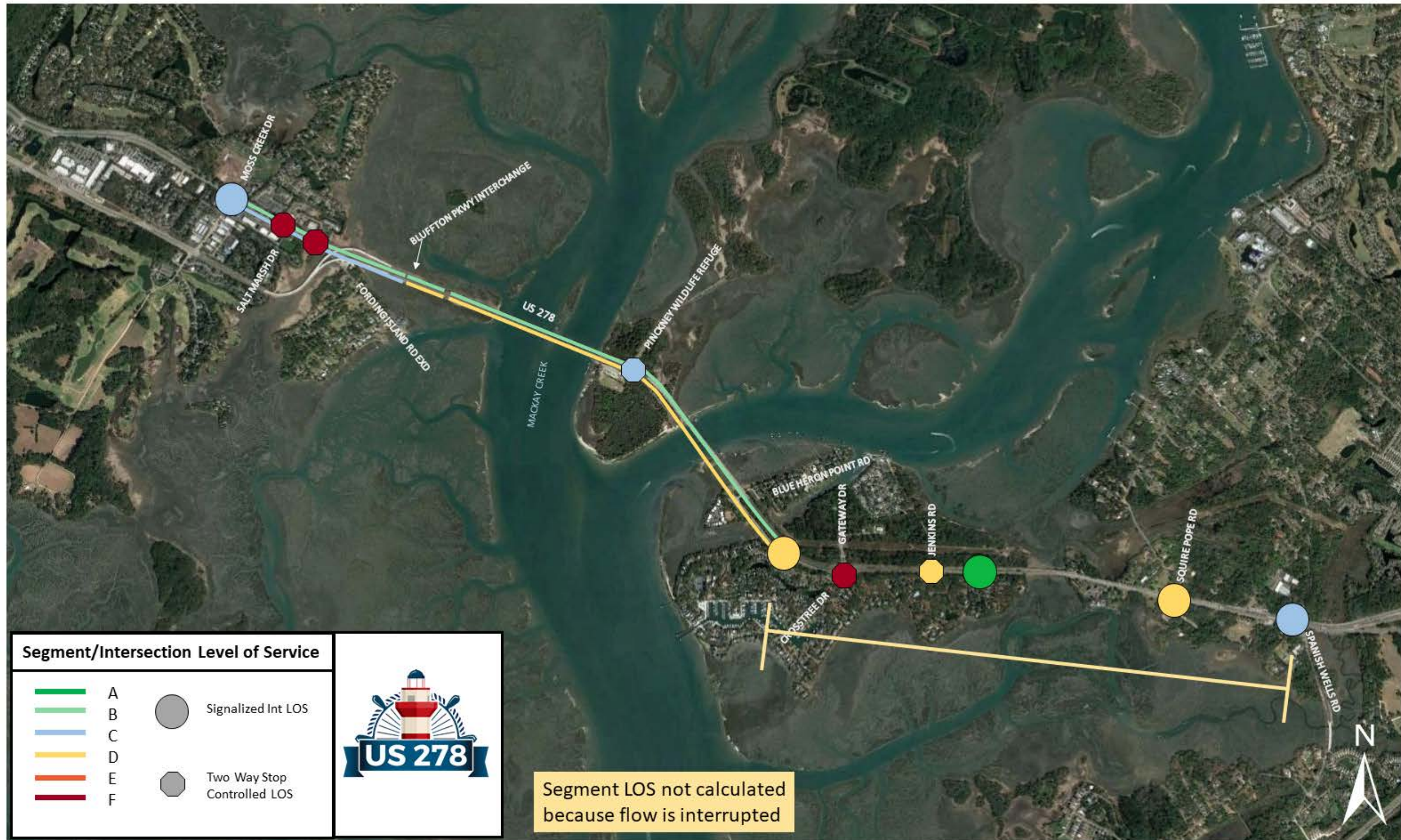
Figure 92: US 278 2045 Reasonable Alternative 3 AM Levels of Service Summary (Includes Jenkins Island Superstreet)
