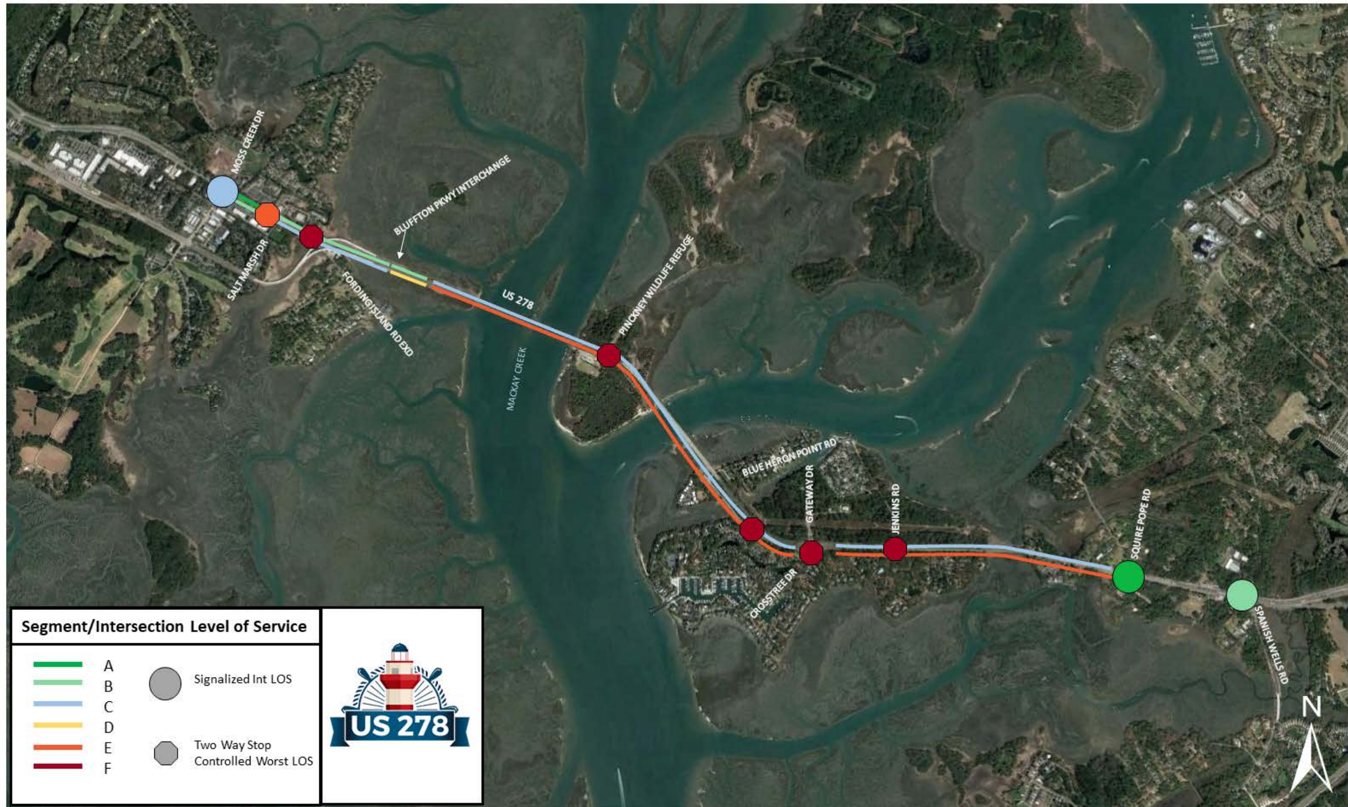
Figure 82: US 278 2025 No Build AM Levels of Service Summary (Excludes Jenkins Island Superstreet)
