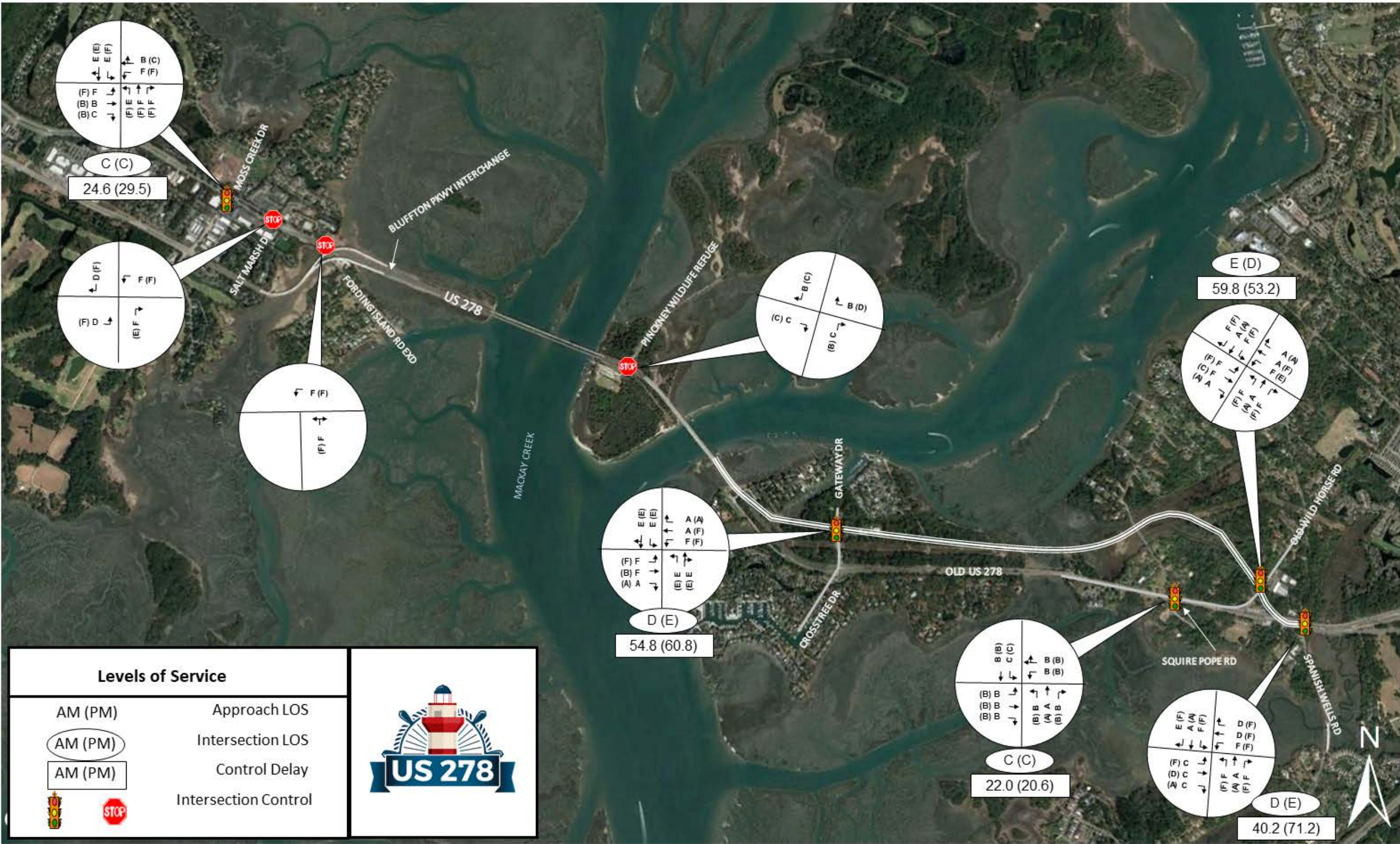
Figure 73: 2045 Reasonable Alternative 5 Intersection Levels of Service
