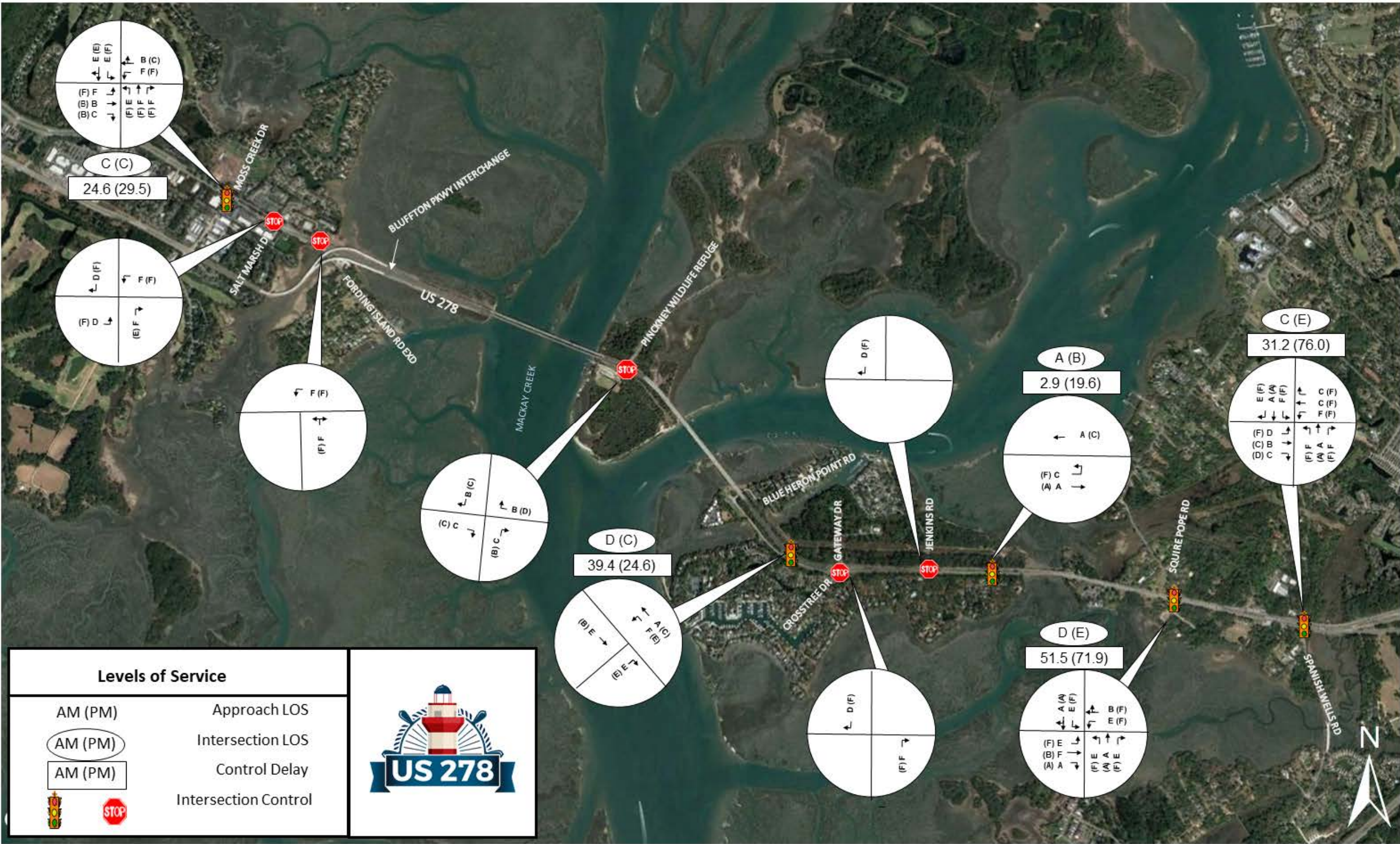
Figure 56: 2045 Reasonable Alternative 1 Intersection Levels of Service
