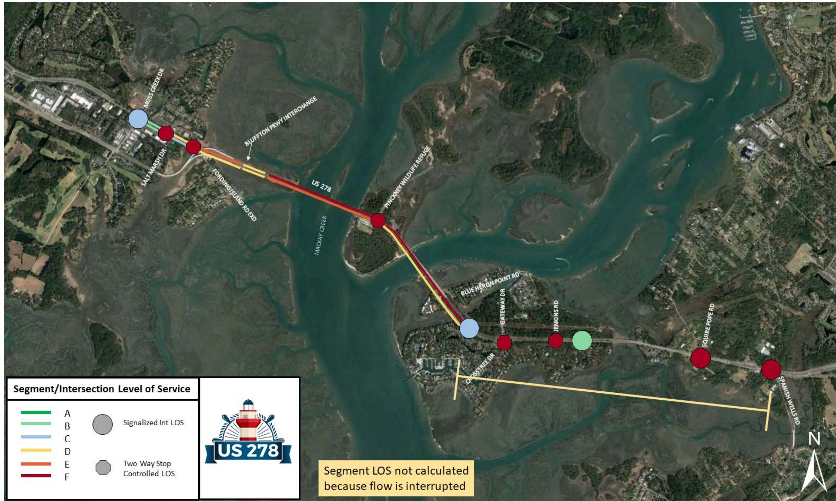
Figure 87: US 278 2045 No Build Plus PM Levels of Service Summary (Includes Jenkins Island Superstreet)
