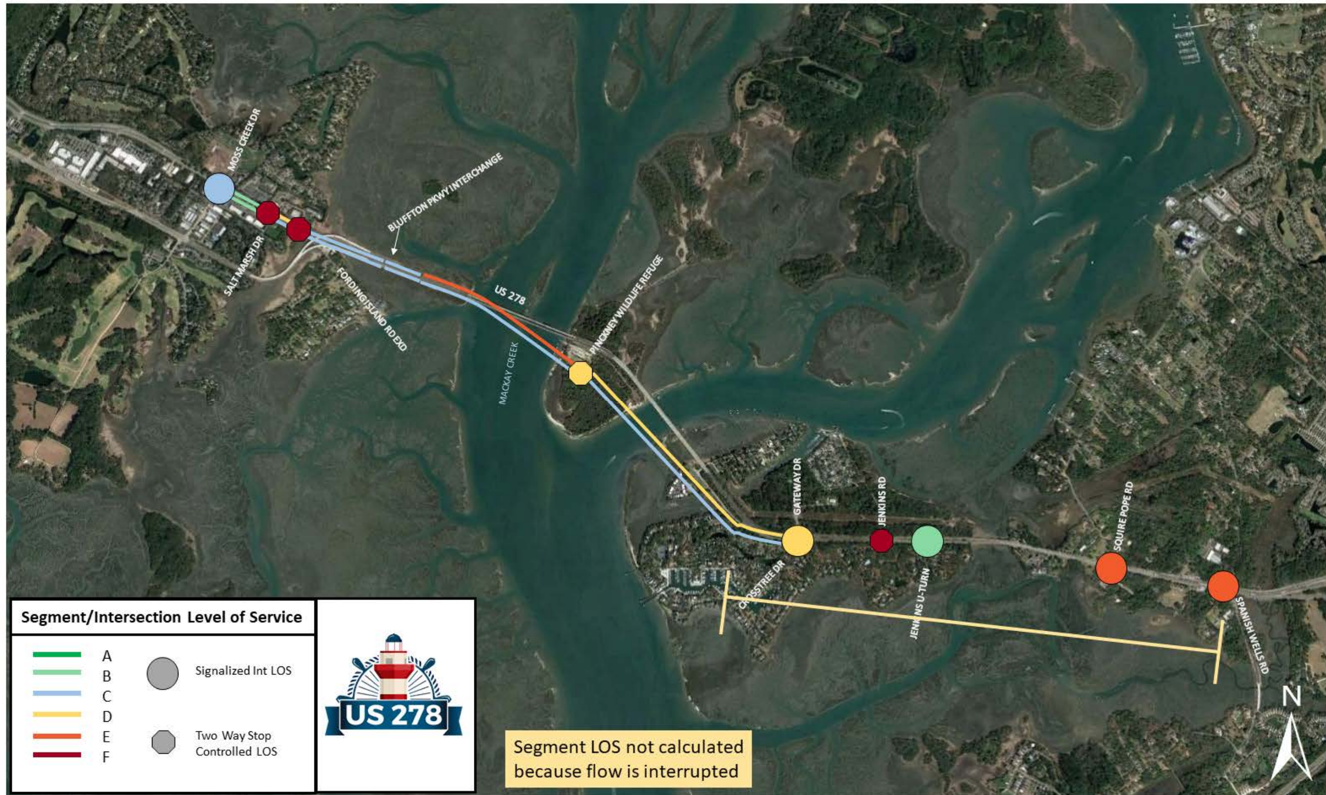
Figure 95: US 278 2045 Reasonable Alternative 4 PM Levels of Service Summary (Includes Jenkins Island Superstreet)
