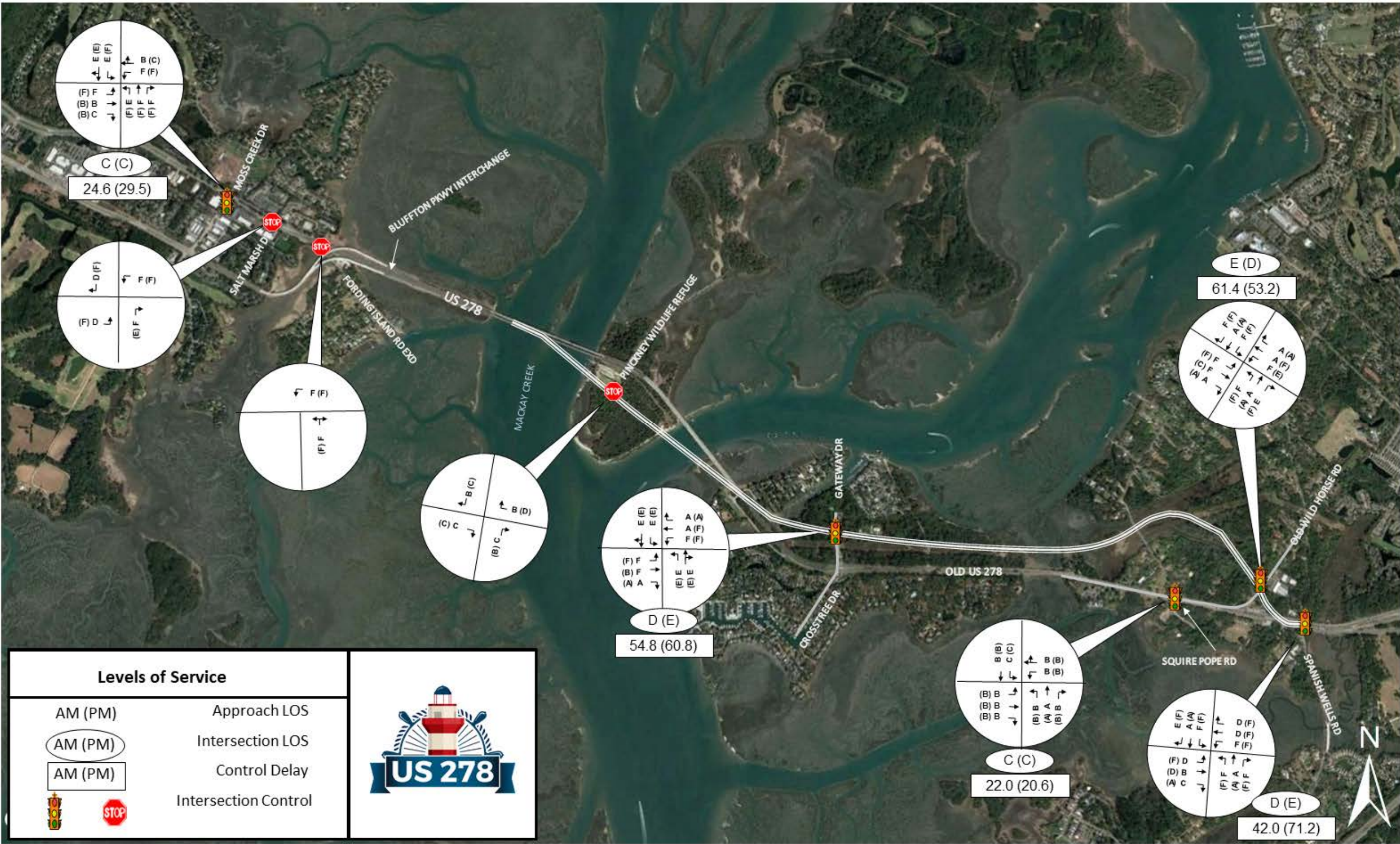
Figure 76: 2045 Reasonable Alternative 6 Intersection Levels of Service
