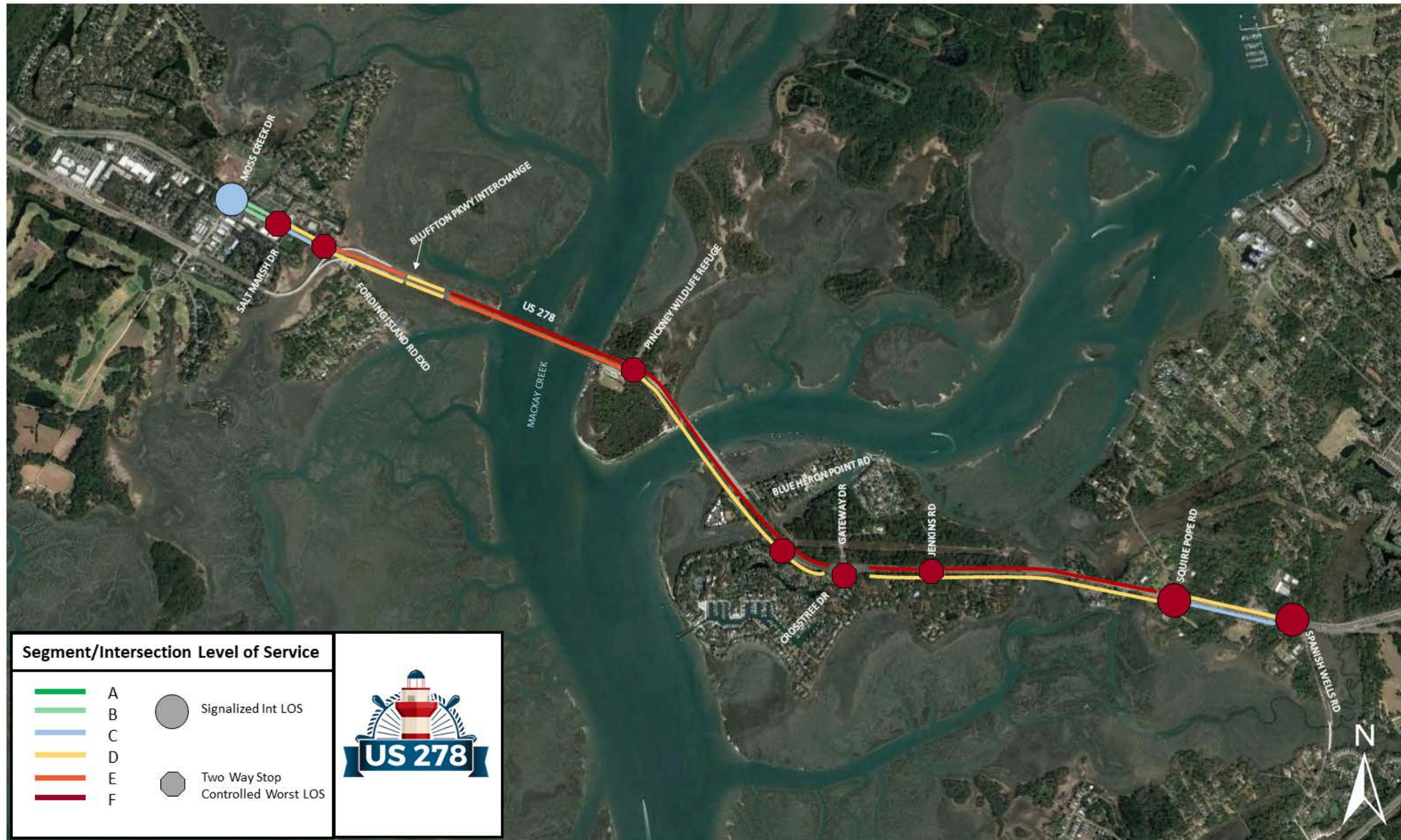
Figure 85: US 278 2045 No Build PM Levels of Service Summary (Excludes Jenkins Island Superstreet)
