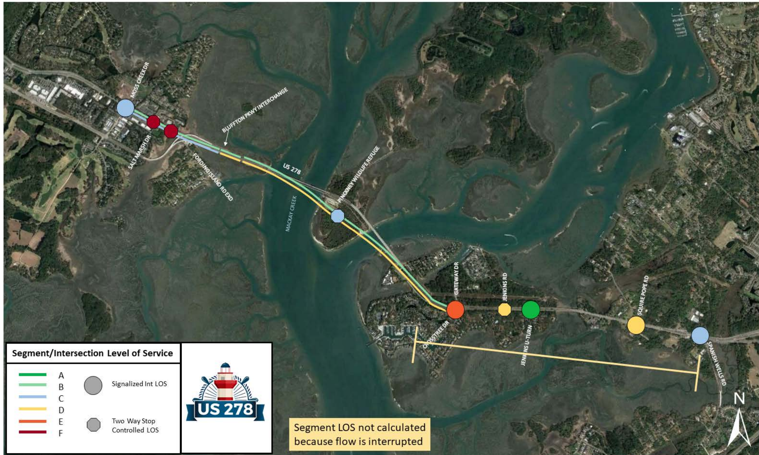
Figure 94: US 278 2045 Reasonable Alternative 4 AM Levels of Service Summary (Includes Jenkins Island Superstreet)
