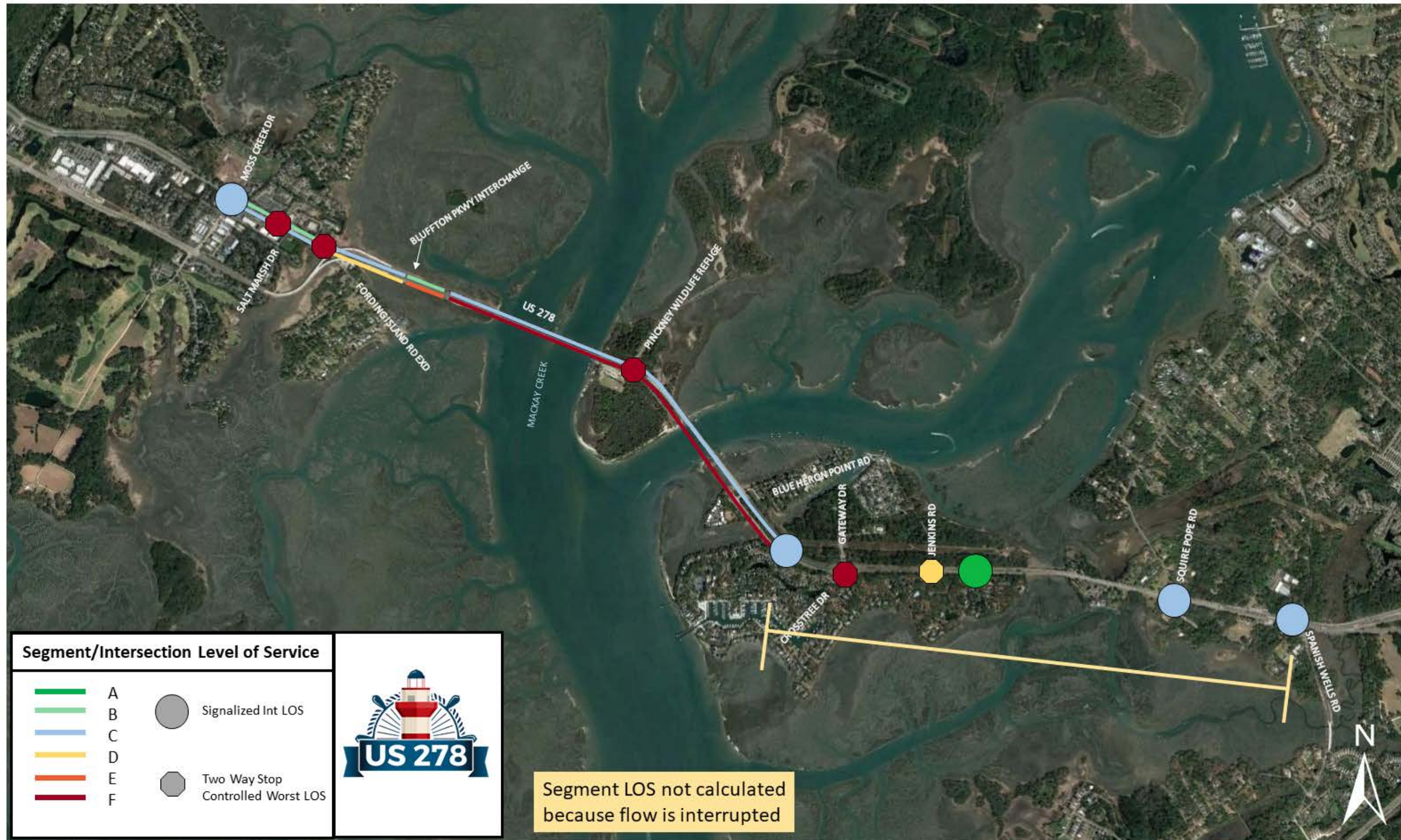
Figure 86: US 278 2045 No Build Plus AM Levels of Service Summary (Includes Jenkins Island Superstreet)
