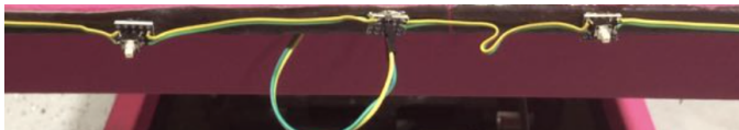
Fig. 4. Bump Sensor Closeup: three on/off buttons that were covered with a long horizontal panel during operation.
