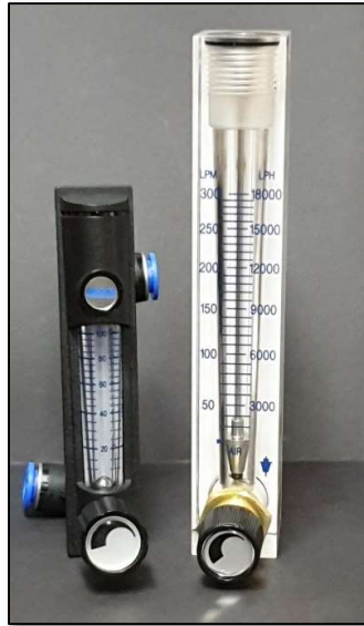
Figure 18: 100 l/m and 300 l/m rotameters
